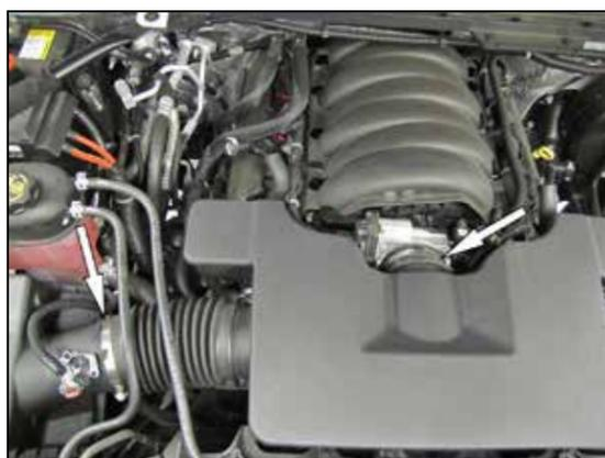
3. Loosen the hose clamps that secure the intake plenum to the throttle body and air filter housing. Then remove the intake plenum from the vehicle.
