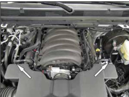
2. Disconnect both crank case quick connect vent lines from the valve covers.
