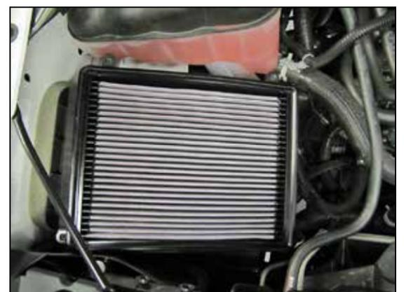
5. Install the AIRAID® air filter into the lower filter housing and then reinstall the upper housing and secure with the factory hardware.
