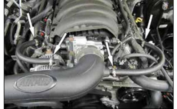
11. Install the crank case vent hose assemblies onto the vent fittings installed into the AIRAID® intake tube and then connect the quick connect fittings to the port on the valve covers.
