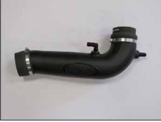
7. Install the provided coupler hoses onto the AIRAID® intake tube and secure with the provided hose clamps.
