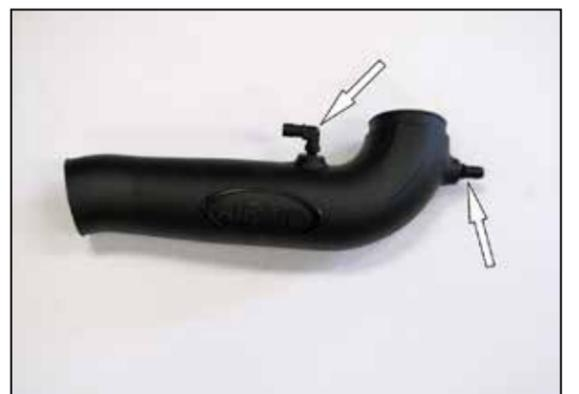
6. Install the provided 90° and straight vent fittings into the AIRAID® intake tube as shown.
