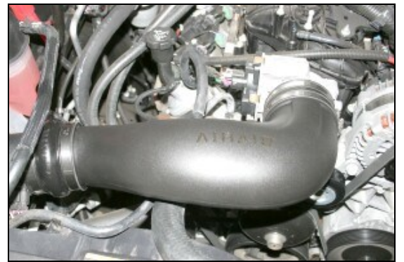
15. Install the Airaid Intake Tube into the Hump Hose first, and then onto the throttle body. Adjust for fit, and tighten the hose clamps. Next install the 3/8" x 14" breather hose (#7) between the 1/4" NPT x 3/8" barbed fitting in the tube, and the factory port on the valve cover.
