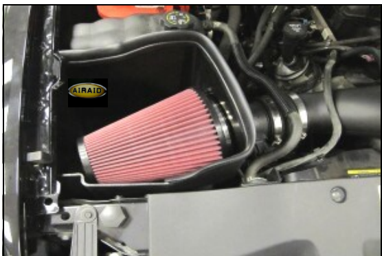
16. Install the Airaid Premium Filter (#1) onto the Air Filter Adapter, and tighten the hose clamp. Next install the provided Weather Strip (#8) onto the top of the CAB. For ease of install, start at the inner fender, and work your way towards the radiator. Reinstall the engine cover.
