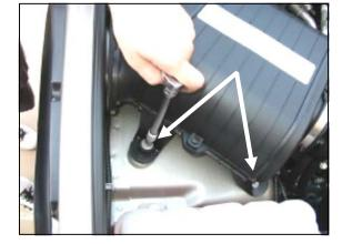
**2.** Using a 10mm socket, remove the three bolts that secure the factory airbox to the inner fender (save for reuse).
