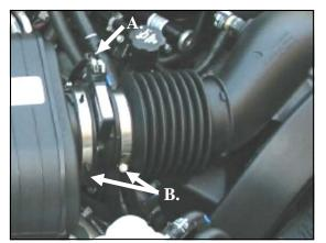
1. <u>Disconnect the negative battery cable.</u>A.) Disconnect the Mass Air Flow (MAF) sensor wiring harness.
