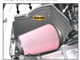
13. Install the Airaid Premium Filter (#1) onto the filter adapter, and tighten the hose clamp. Install the weather strip (#8) onto the Airaid Cool Air Dam. Reconnect the MAF sensor wiring harness. (Note: Start from one corner and work your way around to insure proper alignment of the weather strip.)
