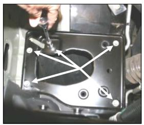
4. Using a 10mm socket, remove the five bolts and mounting plate from the engine compartment.
