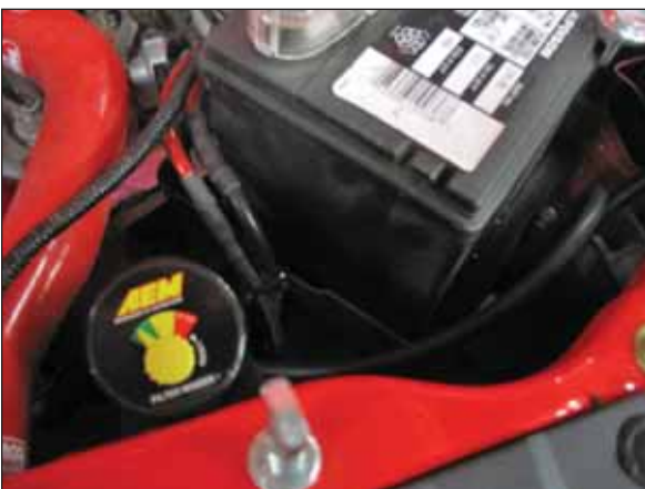
c. Mount under hood in a suitable location using the enclosed bolts and nuts. Alternatively, you may also use zip ties or another method to securely attach the filter minder remote mount assembly to the vehicle. See images for step 3c and 3d as examples for mounting the filter minder
