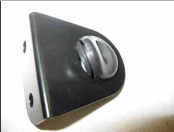
a. Install 3/4" grommet in remote mount bracket.
