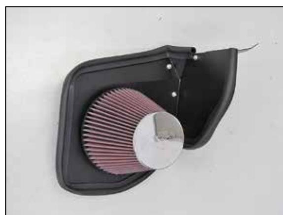
15. Install the K&N® air filter onto the filter adapter and secure with the provided hose clamp.
