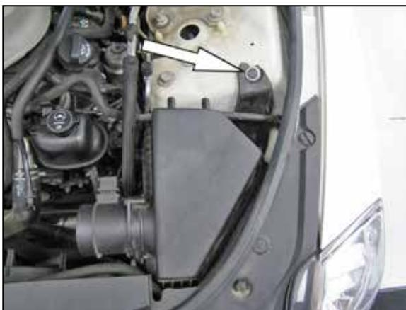
7. Remove the bolt securing the factory air filter housing into the engine compartment.
