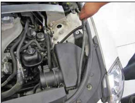
8. Unhook the coolant by-pass hoses and lift them up and over the air filter housing.
