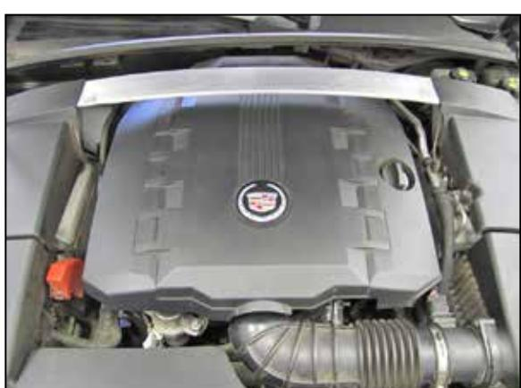
2. Remove the engine oil fill cap and then remove the engine cover. Reinstall the oil fill cap.
