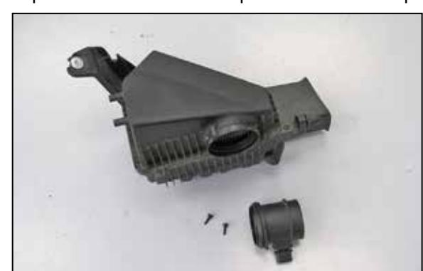
22. Remove the two bolts which secure the mass air sensor housing to the air filter housing and then remove the mass air housing. Remove the O-ring from the mass air sensor housing.
