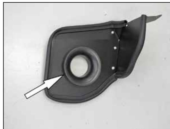
12. Install the filter adapter into the heat shield as shown using the provided hardware.
