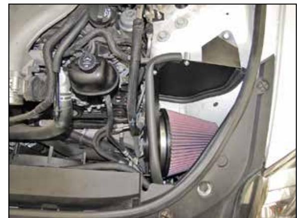
17. Install the heat shield and filter assembly into the engine compartment and secure it the fan shroud with the factory bolt and to the inner fender with the hardware provided.
