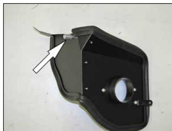
14. Install the 5/8"od aluminum stand-off onto the heat shield as shown.
