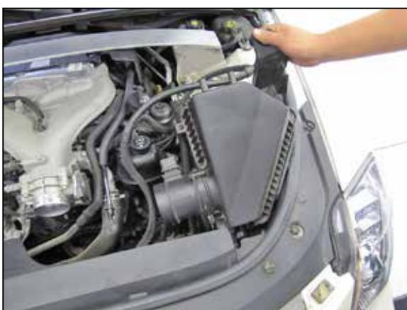
9. Remove the air filter housing from the vehicle.
