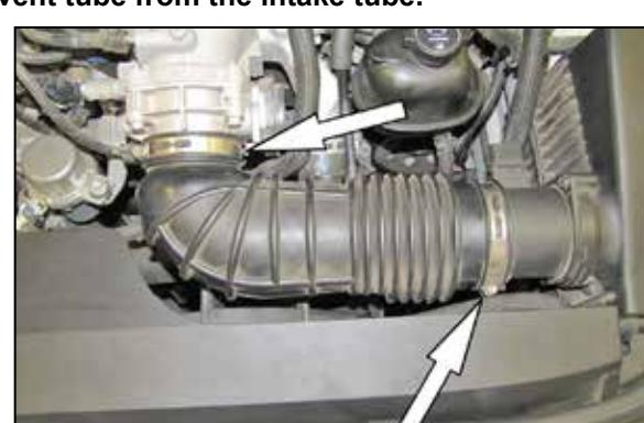
6. Loosen the two hose clamps securing the factory intake hose and then remove the factory intake hose from the vehicle.
