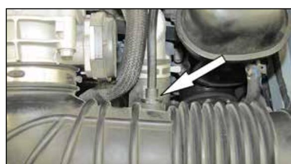
5. Disconnect the crank case vent from the intake tube.
