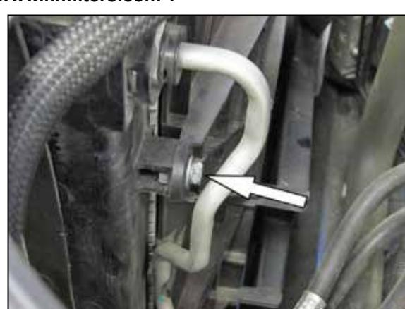
16. Remove the fan shroud mounting bolt shown.
