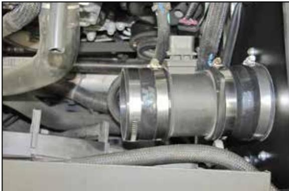
24. Install the provided hose (08632) onto the mass air sensor housing and secure with the provided hose clamp.
