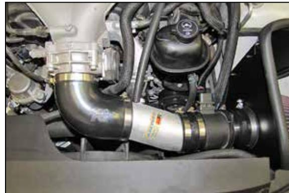
27. Install the tube assembly into the hose at the mass air sensor and align with the throttle body, adjust the tube and elbow hose for best fit and then secure with the provided hose clamps.
