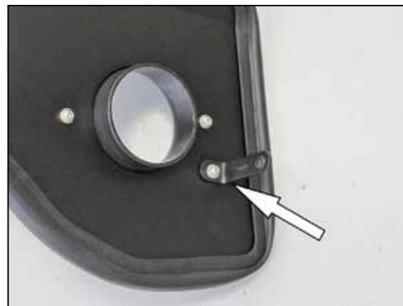
13. Install the "L" bracket (07805) onto the heat shield as shown.
