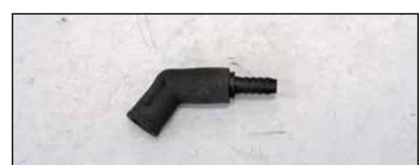
19. Install the provided hose mender into the factory elbow as shown.
