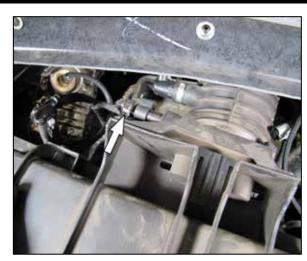
14. Pull the air filter assembly back slightly to expose "F" antenna at the top of the housing. Disconnect the electrical connection of the "F" antenna and then remove the air filter assembly from the vehicle. Remove the two fresh air duct extensions from the vehicle.
