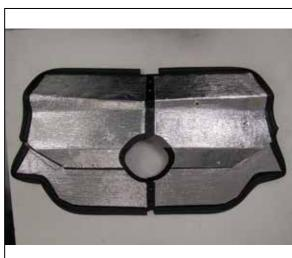
21. Peel the backing off the heat barrier and then apply the barrier to the engine side of the heat shield as shown. After the heat barrier is installed, use a knife or similar tool to cut out all of the mounting holes in the heat shield through the heat barrier.
