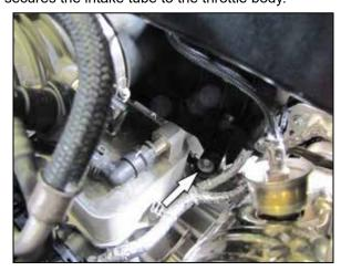
12. Remove the driver's side lower air box mounting bolt.
