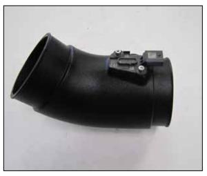
26. Remove the mass air sensor from the factory air filter housing and install it into the K&N intake tube using the provided hardware.
