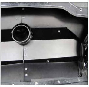
28. Set the intake tube into position but do not secure. Install the passenger side heat shield and align with the mounting bracket. Install all of the mounting hardware loosely before tightening. Reconnect the temperature sensor electrical connection.
