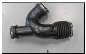
17. Unlock the inlet air temperature sensor and rotate it counter clockwise, remove the sensor from the factory air filter housing.
