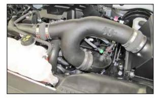
19. Install the K&N® intake tube into the turbo inlet hoses and then into the hose at the throttle body, adjust the tube for best fit and then secure with the provided hose clamps.
