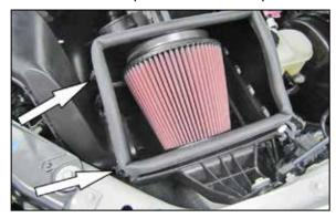
12. Install the heat shield/filter assembly onto the lower air filter housing and secure with the factory retaining clips.
