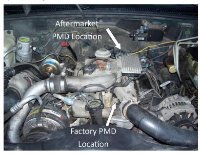
**Note:** An aftermarket PMD may not be in the stock location. Locate, disconnect and plug the JMS PMD into the factory wire harness.
