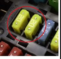
'07 - '10 Shelby Vehicles utilize two fuses. '07 - '12 Shelby GT500 vehicles require the JMS Fuel Pump Wiring Upgrade (p/n: JCA105732)
