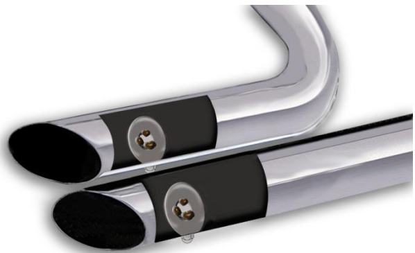
Figure 1 – Exhaust Mod to Reduce Reversion
