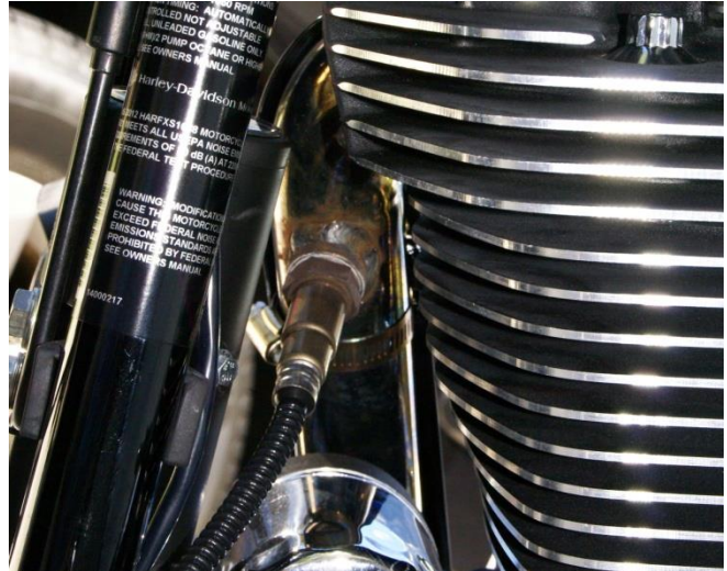
Figure 25 – Typical Rear Sensor Installation
