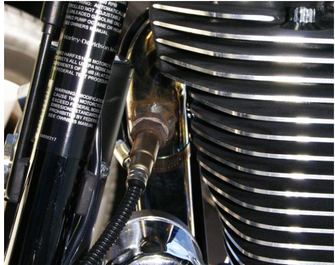
Figure 25 – Typical Rear Sensor Installation
