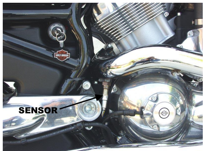
Figure 24 – Typical Rear Sensor Installation
