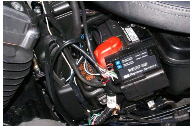
Figure 24 - Typical Sportster® Installation with WEGO IIID Mounted to Side of Battery
