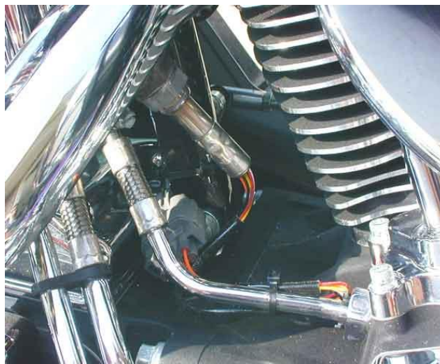
Figure 26 – Typical Sensor Installation
