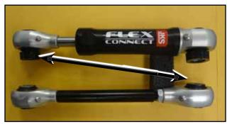
• Adjust the fixed link to be of equal length as the flex connect and lock off the jam nut.
