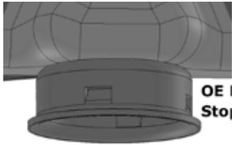
**IMPORTANT:** Internal threads of Jounce Adapter must remain fully engaged with Bump Shock Assembly at all times. Never operate vehicle when more than 3.25" of bump shock threads are exposed as illustrated above.
