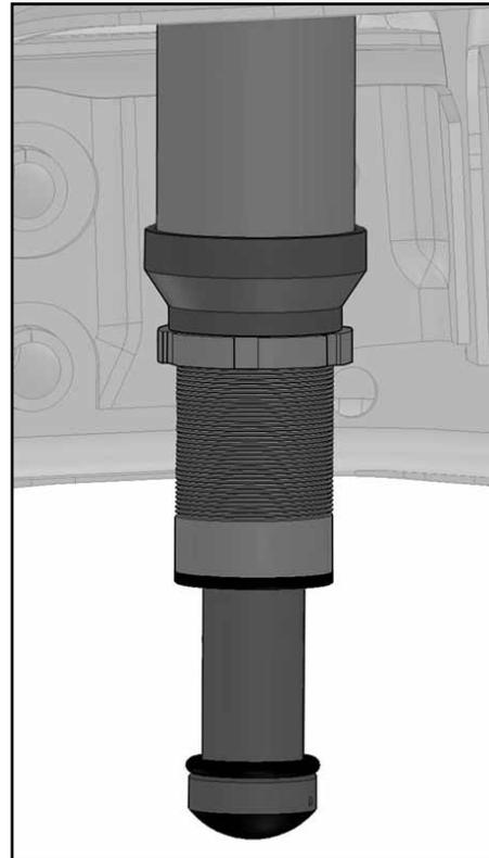
**IMPORTANT:** The suspension must be fully cycled to test for bump shock alignment and interference issues before the vehicle can be safely operated. The bump shock must contact the center portion of the lower spring pad at full compression, and there should be no interference between the bump shock and coil spring at full extension.
