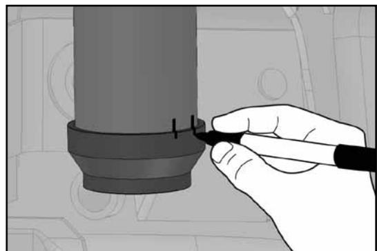
**HINT:** A pair of vertical lines spaced 0.5" apart is used to mark each weld location.
