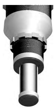
IMPORTANT: The suspension must be fully cycled to test for bump shock alignment and interference issues before the vehicle can be safely operated. The bump shock must contact the center portion of the lower spring pad at full compression, and there should be no interference between the bump shock and coil spring at full extension.
