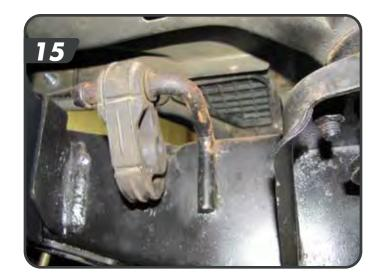
d. Measure in 1-5/8" from the frame rail and make a cut line across the factory shock mount to the crossmember. To avoid a lot of grinding, the crossmember side of the shock mount can be cut just past the weld as shown [16].
