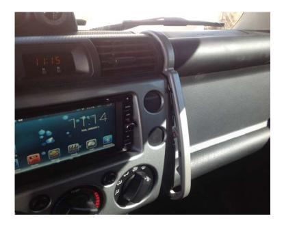
4. Once both trim pieces are removed, you can remove the center dash panel. There is a phillips-head screw on each side of the panel. Remove both screws.
