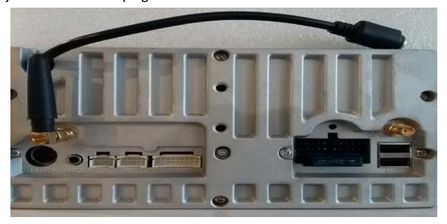
Your Wi-Fi antenna will screw on as shown above. Along with that, your GPS plug in is now on the far right hand side of the FJ1001.
