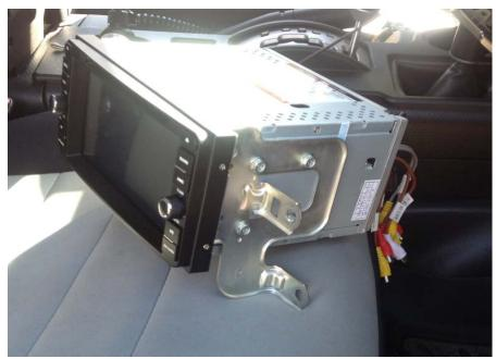
8. Your radio is now ready to install. Determine which harness you need and plug it into the factory harness. You can also install any of the other included cables and accessories such as the microphone, iPod, USB and RCA harnesses that you are going to use. You will also install the Wi-Fi antenna and GPS Satellite antenna.
