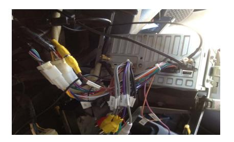
12. As you slide the radio back in, route the wiring behind and under the radio. Slide it in all the way and make sure the brackets fit onto the centering tabs next to the top bracket bolt.
