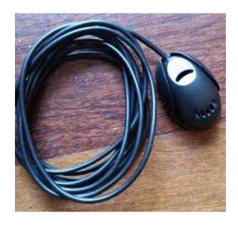
This external mic will work at just about any location, but we do have some recommendations as to placement. Try to keep this mic away from any windows, air vents, or speakers to avoid background sounds or feedback. The external mic will plug into the back of the FJ1001 via a 3.5mm headphone jack plug located just to the left of the RCA pigtail.
