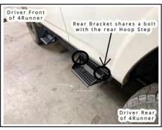
STEP 8 (Tighten **Brackets to**
