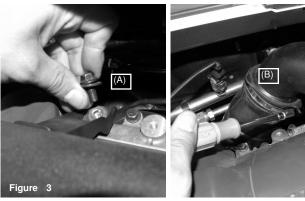
A) With 10mm socket or wrench, loosen and remove the bolt holding in stock intake tube.
