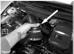
Remove the stock intake tube from vehicle.
