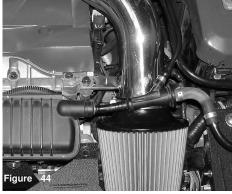
Secure the intake bracket using provided washer and tighten. Connect the vacuum line from step 5.
