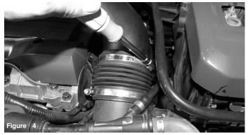
With flat head screwdriver, loosen both clamps on the stock intake tube.
