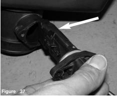
With security bit removal tool or pliers, loosen and remove the 2 screws holding in the MAF sensor and remove.
