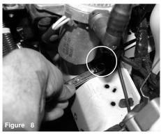
Loosen the vacuum bracket assembly using 8mm nut wrench or socket.
