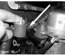
Loosen the bolt holding the harness bracket, and replace with provided M6 vibra mount.
