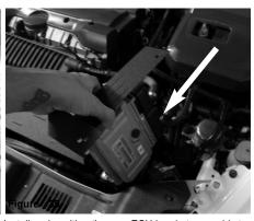
Install and position the new ECU bracket assembly to vibra mount and insert above headlight.
