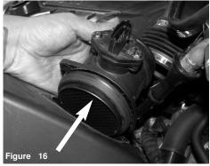
Remove the MAF sensor assembly.
