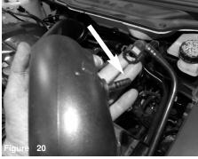
Disconnect the crank case port from the stock intake tube.
