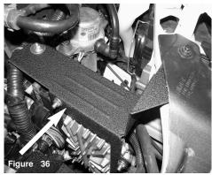
Secure the bracket using the original bolt from step 33. Secure the remaining side using provided M6 nut and washer.
