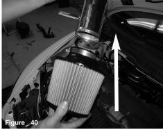
Install the air filter to the intake tube and tighten using 8mm nut driver.
