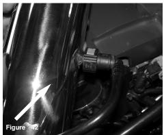
Reconnect the crank case port to new fitting on intake tube.
