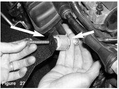
With provided M8 screw and nut, attach and secure the tab on heat shield. Tighten using 13 mm socket or wrench.
