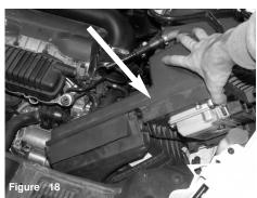
Remove the Complete air box by sliding towards the side of the vehicle. This may require some force. Take caution when removing.
