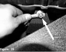
Tighten the stand off stud using provided M6 nut and washer.
