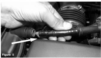
Disconnect the vacuum line from the intake plenum.
