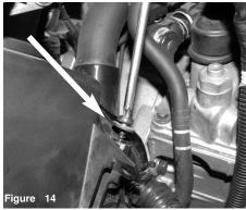
Loosen the screw holding in the ECU harness attached to the air box using t25 torx bit.
