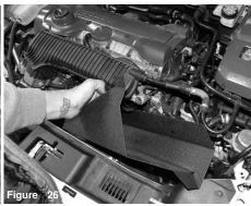
Install the heat shield and position to the factory position.
