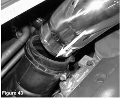
Install the intake tube to factory turbo coupler.
