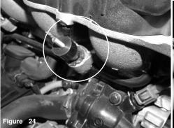
Install the M6 stand off stud, to factory air box grommet. Install the provided spacer to other grommet.
