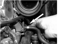
With 10mm wrench, loosen the bolt holding in the stock intake tube bracket.
