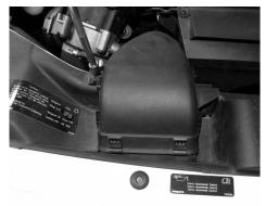
With 8mm socket and ratchet, loosen the 2 bolts hold- Lift and remove the air scoop from the vehicle. ing in the factory scoop.
