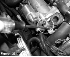
With T25 torx bit, loosen the 2 screws below the air box grommet securing the ECU harness bracket.
