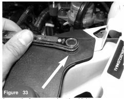
Loosen the 8mm screw above head light.
