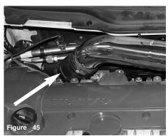
Secure and tighten the intake tube using flat head screwdriver.
