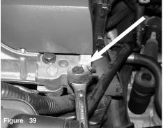
Loosen the bolt on engine for new intake bracket to be secured
