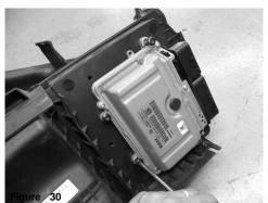
With T25 torx bit, loosen the four screws holding in ECU.
