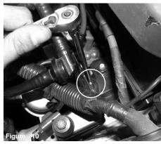
Loosen the remaining bolt holding in the vacuum bracket assembly.
