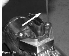
Install the MAF sensor into the new injen intake tube and secure using the provided M4 button head
