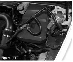
Set aside the complete vacuum assembly on top of battery. This will allow for easier removal of the air box.
