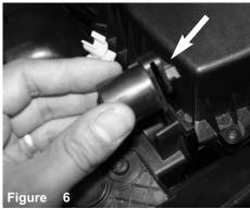
Carefully remove the grommet from air box.
