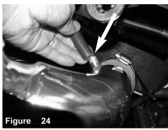
Connect the new hose to the fitting on the tube,
