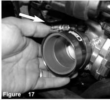
Install the 2-1/4" straight hose with clamps provided to throttle body and tighten on throttle body only.
