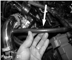
Attach new provided 8mm hose to intake tube and plastic fitting.
