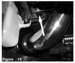
Secure the bracket using provided M8 nut and washer.
