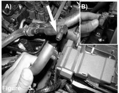
A) Pull back crank case line from fitting. B) Disconnect the MAF sensor harness.
