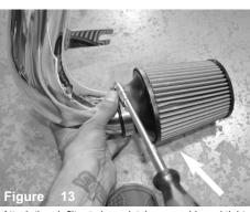
Attach the air filter to lower intake assembly and tighten
