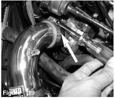
Tighten clamp on throttle body using 8mm nut driver.
