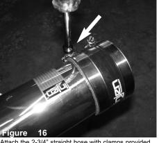
Attach the 2-3/4" straight hose with clamps provided to upper intake tube assembly and tighten on tube only.
