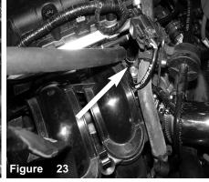
Route the hose through engine compartment if desired
