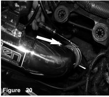
Position best possible fit and tighten remaining clamps using 8mm nut driver.
