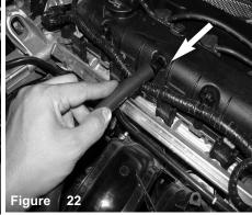
Install provided 10mm hose to crank case on engine side.
