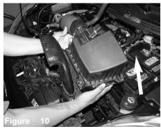
Carefully lift and pull out air box.
