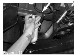
For easier installation, you can carefuly lift front of vehicle. From under neath vehicle or from up top, attach M8 male/female vibra mount to stud on frame next to washer resovoir and secure.
