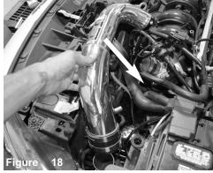
Install upper intake tube assembly and position to lower intake tube and throttle body. Connect the 2 intake tubes together
