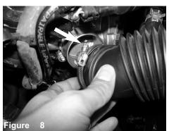
Pull back intake tube from throttle body.
