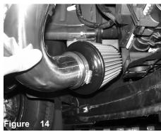
Install the lower intake assembly into cut out next to washer resovoir and radiator. Position the bracket on intake tube to vibra mount.
