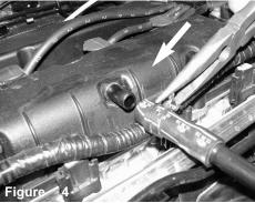
Disconnect the electrical MAF sensor harness.
