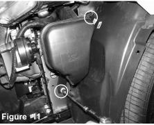
Loosen the 2 screws holding in the resonator box.
