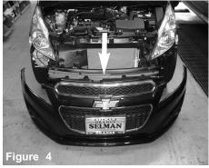
Removal of front bumper cover is necessary. remove top and bottom screws of bumper cover and side screw under head light near fender line.
