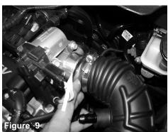
Pull back the intake tube from the throttle body.
