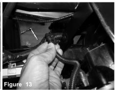
Locate the harness clip connected on frame near head light and remove, this will be used for the vibra mount.
