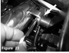
Now tighten the vibra mount using 10mm wrench.
