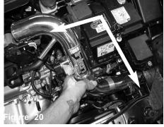
Install the intake tube into vehicle and position to throttle body and bracket to vibra mount.
