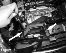
Loosen the screw holding in the factory snorkel. Remove push clip also.
