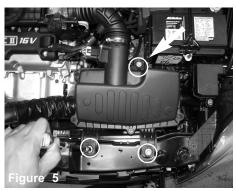
With 10mm socket and ratchet, loosen the 3 screws holding in the stock air box.
