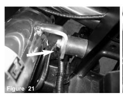
Secure the bracket using M6 nut and fender washer. Do not tighten.
