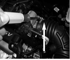
Loosen the clamp on the throttle body using 7mm nut driver.
