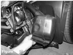
Carefully remove the resonator box out of vehicle.
