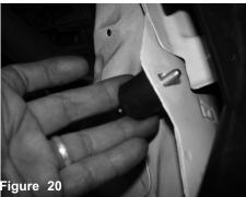
Attach the vibra mount to the front of the vehicle on square hole cut out on radiator support.
