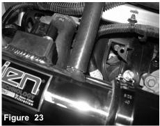
Connect crank case line to intake tube.
