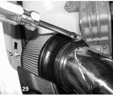
Install the high flow filter to intake tube and tighten using 8mm nut driver.
