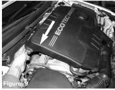
Lift up engine cover and remove from vehicle.
