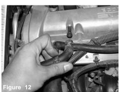
With pliers pull back crank case line from engine.
