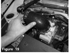
Install the elbow hose with clamps provided to the throttle body. *Make sure the short side of hose is on the throttle body.*
