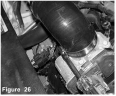
Tighten the clamp on throttle body using 8mm nut driver.
