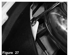
Tighten both nuts on vibra mount using 10mm
