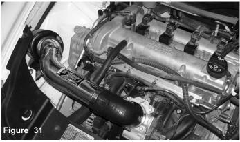
Congratulations! You have just completed the installation of this intake system. Periodically, check the alignment of the intake, normal wear and tear can cause nuts and bolts to come loose. Failure to check the alignment and adjust the intake can cause damage that will void the warranty.
