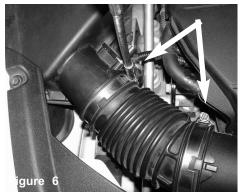
Loosen the 2 clamps using 8mm nut driver.
