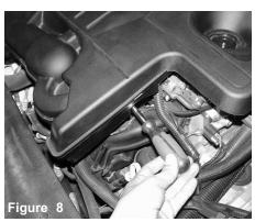
With long 8mm nut driver, loosen the clamp under the engine cover on throttle body.
