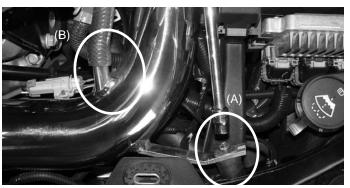
Using a 10mm socket or nut driver screw the 6mm flange nut and fender washer on the vibra-mount stud (A). Take the 7 1/2" 12mm reinforced vacuum hose and one end over the crankcase port and the other end over the 5/8" port on the intake (B).
