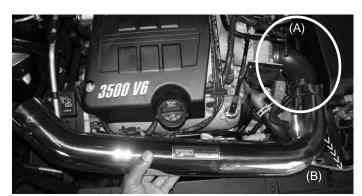
Take the primary intake and press the end with the 90 degree bend into the elbow on the throttle body (A). Once the intake has been pressed into the silicone, align the bracket on the intake to the vibra-mount stud (B). Page 2 of Part# SP7030
