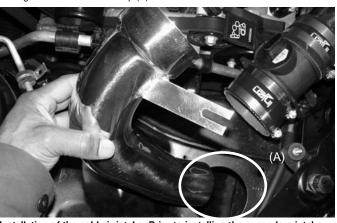
Installation of the cold air intake- Prior to installing the secondary intake press the vinyl trim around the inside diameter of the resonator opening (A). Once the vinyl trim is in place, lower the secondary intake into the resonator opening.
