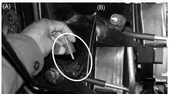
Take the vibra-mount and screw it into the pre-tapped metal bracket located on the front passenger side, above the head lamp (A). The vibra-mount will set flush on the metal bracket (B).
