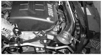
Press the 3-1/4" step hose (black hose) over the end of the primary intake, use two medium clamps on the straight hose. Tighten the clamp on the intake side prior to moving on to the next step (A).
