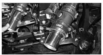
when using the short ram, press the secondary step intake and press the 3 3/8" end into the mass air sensor hose (A). Align the intake bracket to the vibramount stud (B). Once the bracket has been aligned adjust the intake for best fit and tighten the clamp on the mass air flow sensor (C).
