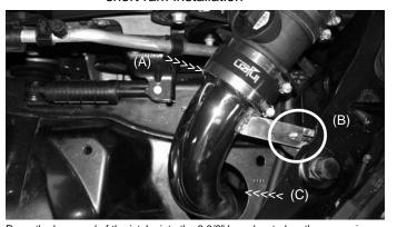
Press the large end of the intake into the 3 3/8" hose located on the mass air sensor (A). Align the intake bracket to the vibra-mount stud (B). Keep proper clearance around the resonator opening. The intake should not touch any area along the edge of the resonator opening (C).
