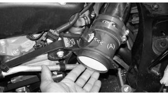
Take the directional mass air flow sensor and press the outlet end into the 3 1/8" hose located on the primary intake. Locate the female harness connector facing the firewall (A)
