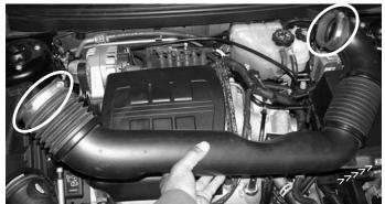
Loosen the clamps and m6 bolt to remove the stock air intake duct that connects the stock air box to the throttle body.
