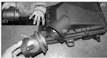
Loosen the m6 bolts that secure the stock air box to the mounting points. Remove the air intake box from the engine compartment (A). Once the stock air box has been removed the engine compartment loosen the bolts the hold the mass air flow sensor to the stock air box (B). Remove the O-ring from the mass air flow sensor which will not be used in this installation (C).
