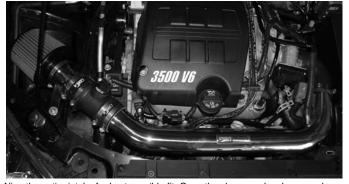
Align the entire intake for best possible fit. Once the clearance has been made through out the length of the intake continue to tighten all nuts, bolts and clamps. The short ram intake is now fully installed.
