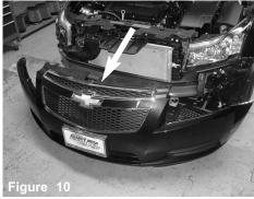
Carefully remove the bumper cover, this requires 2 Remove the air box snorkel guard from the vehicle. 10mm bolts on top, push-clips, and t-25 screws located on the bottom of the vehicle. This is required for the cold air installation.
