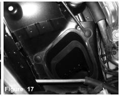
Remove the 2 clips holding in the plastic auxilary inlet.
