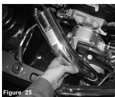
Install the lower intake assembly into the vehicle and position the bracket to the vibra mount.
