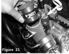
Attach and install the step hose to the turbo with
