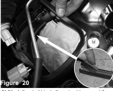
A) Attach the vinyl trim to the cut out to prevent the tube from vibration on frame. B) Cut provided 8mm hose with a blade down the center and install to the A/C line to prevent any touching between the intake tube and A/C line.
