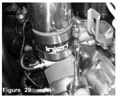
Position the intake for the best fit and tighten all clamps on intake usign 8mm nut driver
