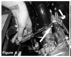
Loosen the clamp on the turbo using 7mm nut driver.
