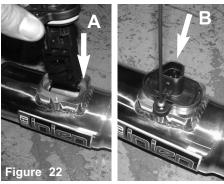
A) Install the MAF sensor into the new intake tube. B) Secure and tighten using provided M4 button head clamps provided and tighten on the turbo side only. screws.
