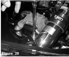
Position the intake for the best fit and tighten the vibra mount using the remaining washer and nut and tighten using 10mm socket or wrench.
