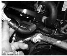
If you want, you can remove the drain plug from the vehicle's frame. This will not plug into the new intake system.
