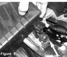
Pull back the front grommet from the bottom of the air box.
