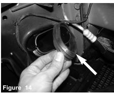
Remove the gasket from the resonator.
