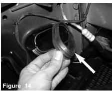
Remove the gasket from the resonator.
