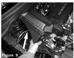
Lift up stock intake and remove from vehicle.
