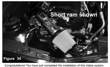
Periodically, check the alignment of the intake, normal wear and tear can cause nuts and bolts to come loose. Failure to check the alignment and adjust the intake can cause damage that will void the warranty.
