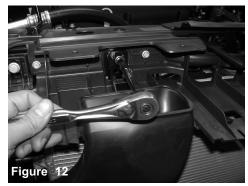
Loosen the bolt holding in the air box snorkel using 10mm socket and extension.
