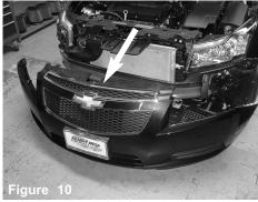
Carefully remove the bumper cover, this requires 2 10mm bolts on top, push-clips, and t-25 screw slocated on the bottom of the vehicle. This is required for the cold air installation.
