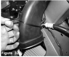
Re-install the air box snorkel and secure the bottom end of snorkel with provided zip ties to prevent from moving.
