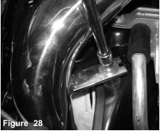
Position the intake for the best fit and tighten the vibra mount using the 2 remaining washer and nut and tighten using 10mm socket or wrench.
