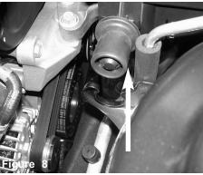
Pull back the second grommet on the back of the air box.
