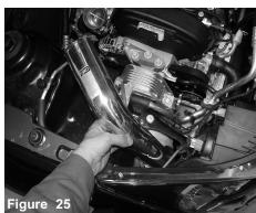
Install the lower intake assembly into the vehicle and position the bracket to the vibra mount.
