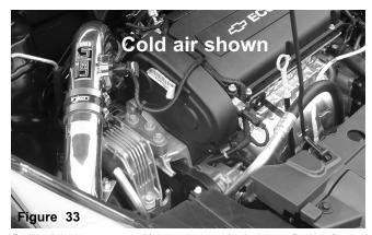
Re-install the bumper cover. Make sure everything is tighten. Position for best possible fit. For Short ram, remove the lower intake assembly and attach the filter to the upper intake tube assembly and secure. See figure 34.
