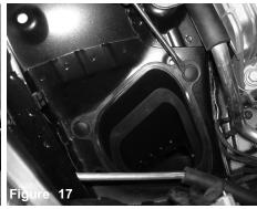
Remove the 2 clips holding in the plastic auxiliary inlet.
