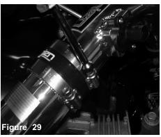
Position the intake for the best fit and tighten all clamps on intake usign 8mm nut driver
