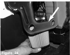
Place the filter in the resonator position next to the frame.
