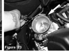
Attach and install the step hose to the throttle body with clamps provided and tighten on the throttle body only.
