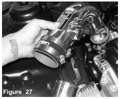
Install the upper intake tube assembly with straight hose and clamps provided and connect the 2 tubes together.
