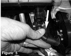
Pull back drain plug from the bottom of the air box.
