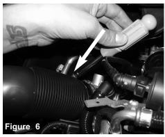
Loosen the clamp on the throttle body using 7mm nut driver.
