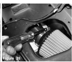
Tighten the filter and secure on the intake tube using 8mm nut driver.
