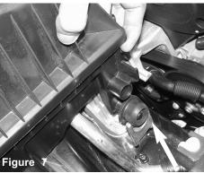
Pull back the grommet from the bottom of the air box.
