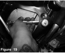
Attach the vibra mount to the hole used to hold in auxilary inlet. Secure using provided nut and washer and tighten using 10mm wrench.
