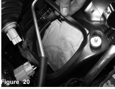
Attach the vinyl trim to the cut out to prevent the tube from vibration on frame.
