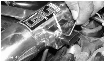
An allen wrench is used to fastened the m4 bolts to the machined adapter.
