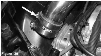
The silicone hose is pressed over the end of the primary intake, a power band is used to secure the silicone hose over the intake end.
