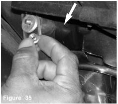
The new filter is aligned to the end of the intake and pressed over the intake.
