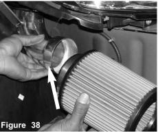
As soon as the filter stops are butted up against the filter stop, continue to tighten the filter clamp.
