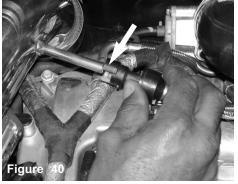
The vacuum clip is pressed over the machined vacuum port.
