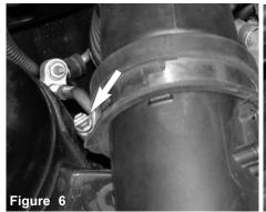
The turbo air inlet clamp is loosened in order to separate the air box from the air intake duct.
