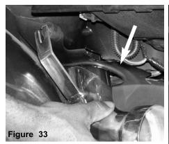
Once you have aligned the secondary intake to the vibra-mount, continue to tighten the m6 nut. Page 4 of Part# SP7027
