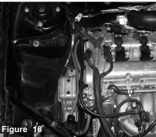
The air box cleaner and air duct is removed from the engine now removed.
