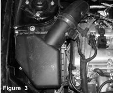
The stock air box and air duct to be removed. Prior to the installing, disconnect the negative battery terminal. The front bumper is removed prior to starting.
