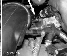
The lower turbo air inlet clamp is now loosened as shown above.
