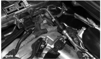
Check the harness clip and vacuum lines for proper fitment. Make sure there is good contact between the harness clip and mass air flow sensor, check for any possible vacuum leaks in the vacuum connections.
