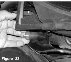
The vibra-mount is inserted into the bumper support frame. The nut and washer is lowered from the inside.
