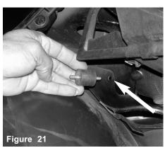
The male vibra-mount is inserted into the pre-drilled hole located on the passenger side bumper support.
