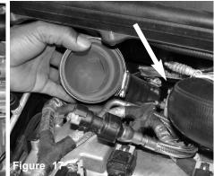
The silicone elbow is now lowered into the engine compartment and over the turbo inlet. The clamp over the turbo is now semi-tightened.
