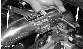
Once you have aligned the intake bracket to the vibra-mount , continue to press the intake into the hose over the throttle body.
