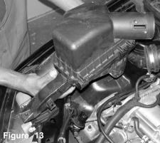
Once all three bolts and clamp has been removed or loosened, continue to pull the air box cleaner from the engine compartment.
