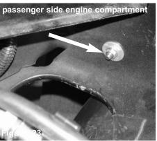
The m6 flange nut is placed over the vibra-mount stud located on the opposite side of the fender or inside of the engine compartment.
