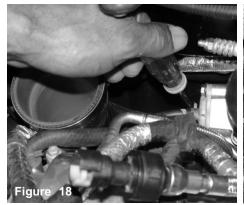
The clamp is tightened over the silicone hose.
