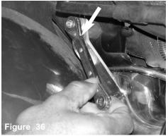
A ratchet or nut driver is used to fasten the m6 flange nut.
