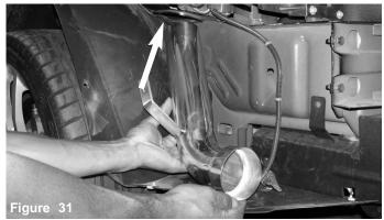
The secondary intake is inserted into the bumper corner and into the engine compartment.
