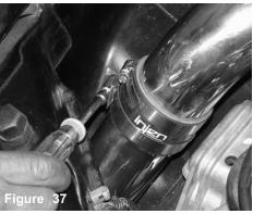
The mass air flow sensor is slowly lowered into the machined sensor adapter.
