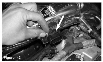
Once the sensor is secured in place, continue to use the m4 bolts in kit to fasten the sensor in place.
