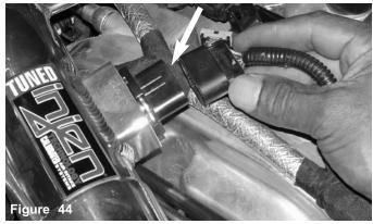
Once you have fastened the m4 bolts, continue to press the electrical harness clip over the mass air flow sensor.
