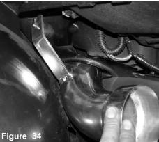
The secondary intake is now installed and secured to the vibra-mount.
