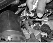
The vacuum port connector is removed from the air duct port as shown above.
