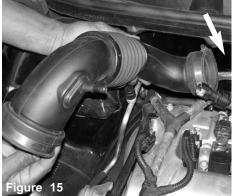
The lower air duct is now pulled out from the engine compartment.
