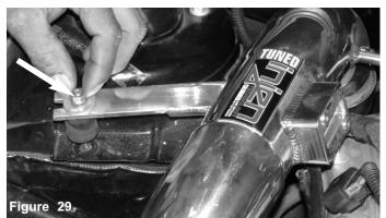
The m6 flange nut is tightened.
