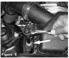
The second flange nut is loosened and removed.
