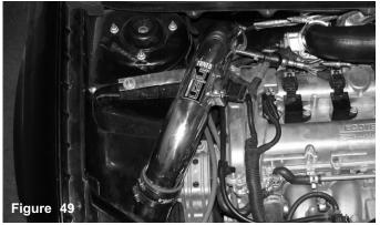
Congratulations! You have just completed the installation of the best air intake system made. Prior to driving, start the engine, and listen for any air leaks, rattling or vibration. Allow 5 to 10 minutes for the ECU to adjust to the added volume or air created by the cold air intake.
