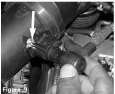
The two bolts are loosened and removed from the mass air flow sensor housing.
