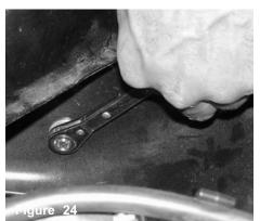
The m6 flange nut is tightened over the vibra-mount stud.
