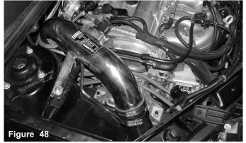
Check the connection of the intake bracket to the vibra-mount and the alignment of the primary and secondary intakes. Everything should be properly aligned to prevent damage to the cold air intake.
