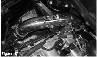
Periodically, check the fitment of both intake systems. Normal driving conditions may loosen nuts, bolts and clamps causing intakes to shift resulting in damage to automotive parts.
