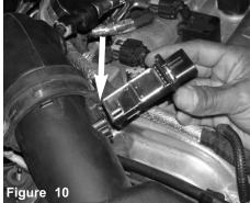
Once you have removed both bolts, continue to pull the mass air flow sensor from the sensor housing.
