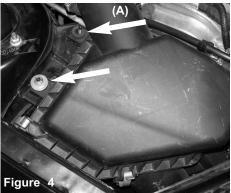
The two m6 flange nuts are removed. The top m6 flange nut has already been removed (A)
