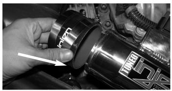
To convert your intake system into a cold air intake take the 3" straight hose and press it over the end of the primary intake. Use two clamps from the kit to place them over the hose and tighten the clamp on the intake.
