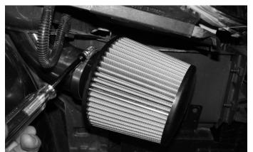
Press the Injen filter over the end of the secondary intake. Press the filter over the intake until it butts up against the stops built inside of the filter neck. Do not over run the intake end past the filter stop, this may obstruct the air flow if incorrectly installed.
