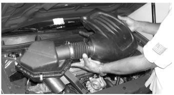
Once the stock clamps have been loosened remove the entire air intake box from the engine compartment.
