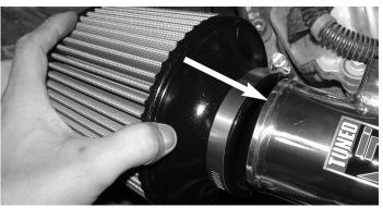
Once the primary intake has been set in place semi-tighten the clamp on the intake side. Take the filter and press it over the end of the intake and tighten the clamp on the filter neck.
