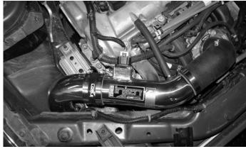
Once the cold air intake has been installed align the entire intake for best possible fit. Make sure there is no rubbing parts along the length of the intake then continue to tighten all nuts, bolts and clamps. Periodically, check the alignment to avoid any damage to the intake system.
