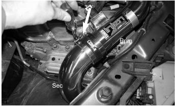
While the intake bracket is located on the vibra-mount stud press the top end of the secondary intake into the 3" hose on the primary intake. Once both intakes have been aligned to each other continue to semi-tighten the clamp.
