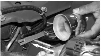
Once the secondary intake has been inserted into the resonator opening align the bracket to the vibra-mount stud.
