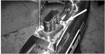
Take the MAF sensorremoved earlier from the stock air intake box and press it into the machined adapter. Use the stock sensor screws to reattached the MAF into the machined adapter. Secure the MAF sensor using the 2 M4 screws provided.
