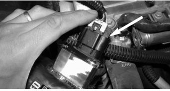
Locate the stock harness clip and plug it into the MAFS. Press the harness into the sensor until you here it snap in place.
