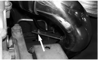
Take the 6mm flange nut and fender washer and secure the intake bracket to the vibra-mount stud.
