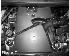
Loosen the 3 bolts holding in the air box using 8mm socket or nut driver.
