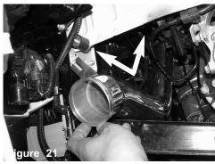
Install the lower intake assembly into the bottom of the vehicle and position to the upper intake assembly and bracket to the vibra mount from step 18A.
