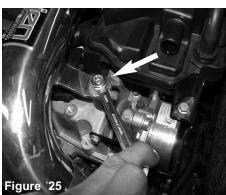
Secure the bracket on upper intake tube assembly using 10mm wrench.
