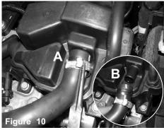
A) With pliers carefully remove the safety clamp on the Carefully jack the front driver side of vehicle, and crank case line.
