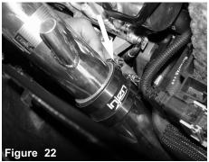
Connect the upper and lower intake tubes. Tighten using 8mm nut driver. Keep snug in case you need to re-position.
