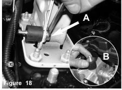
A) Secure using provided M6 nut and washer. Tighten using 10mm wrench. B) Install the vibra mount to the fitting on the engine under the crank case CCV box. (stock air box mounting insert)
