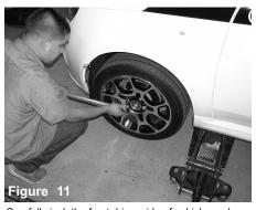
loosen the bolts on the front wheel and remove. This will allow for easier installation. Note: Make sure the vehicle is secure!
