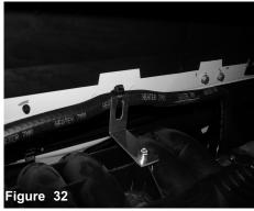
Snug fit the coolant line to the bracket.
