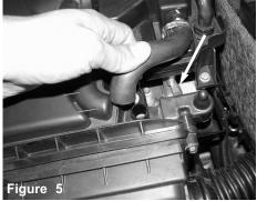
Pull out the crank case line from the air box.
