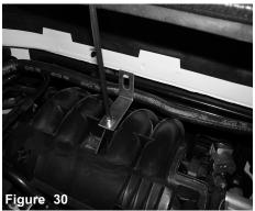
Secure using provided M6 button head screw.
