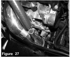
Attach the 15.9mm hose to the fitting on the intake tube
