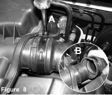
A) Loosen the clamp on the air box only.
