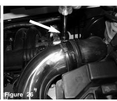
Position for the best possible fit and clearance. Tighten all clamps using 8mm nut driver.
