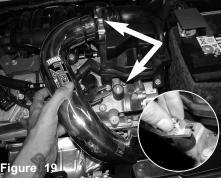
A) Install the upper intake tube assembly and position to the stock intake hose and bracket to the vibra mount. B) Secure bracket using provided M6 nut and washer. Do not tighten.
