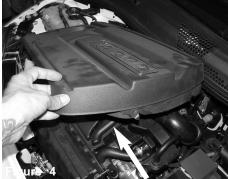
Lift up the engine cover, and remove.
