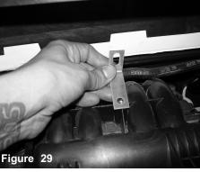
Place the stainless bracket to the insert on the back close to the firewall. (stock air box insert)
