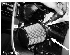
Install the air filter and tighten using 8mm nut driver.
