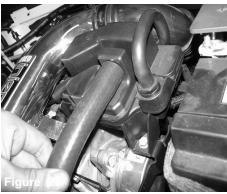
Now install to the fitting on the CCV crank case box.
