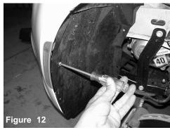
Loosen the screws holding in the splash guard.
