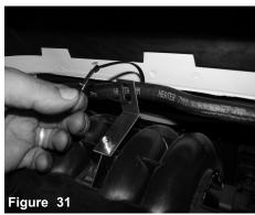
Posiiton the coolant line to the back of the bracket, and secure using the provided zip tie.
