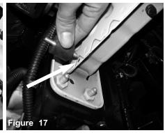
Install the vibra mount to the hole on the front of vehicle frame.
