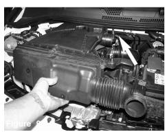
Pull out the complete air box assembly. Make sure the coolant line is apart from the back of the air box.
