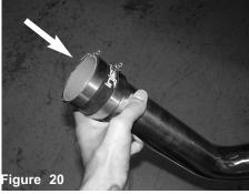
Attach the hose with clamps to the lower intake assembly.
