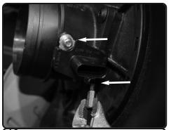
13. With provided T20 torx security bit, loosen and remove MAF sensor. Save screws for later install. **Note: Keep sensor in same direction.**
