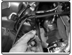
**20.** With provided zip ties, secure the MAF sensor and headlight harness. Re-install the plastic cover and secure.
