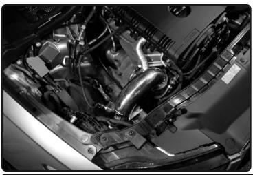
Congratulations! You have just completed the installation of this intake system. Periodically, check the alignment of the intake, normal wear and tear can cause nuts and bolts to come loose. <u>Note: Check clearance and adjust if needed! Failure to check the alignment and adjust the intake can cause damage that will void the warranty. Injen Technology is not responsible for any damages caused by/from improper installation.</u>
