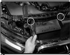
**5.** Locate the 2 bolts holding in the front air scoop and loosen and remove using T25 torx bit.
