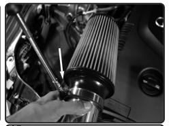
**15.** Install the filter to the intake tube and secure using 8mm nut driver.
