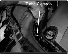
**8.** Loosen the clamp on the turbo using 7mm socket with ratchet.
