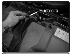
**3.** Carefully remove the push clips using flat head or panel clip removal tool.
