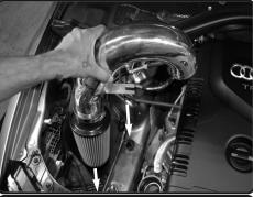
**16.** Install the intake tube assembly. position the bracket to the washer and the intake tube to the step hose.
