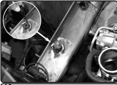
**10.** Now install the provided M6 stand off stud to the grommet that air box mounted to on frame. This will seat in the grommet.
