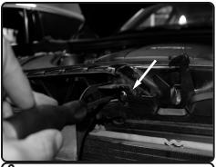
**6.** The other bolt will be located bhind first bolt holding in plastic shroud. This will now have access to the remaining bolt.
