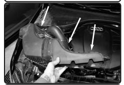
**9.** Carefully lift up and remove the entire air box assembly out of vehicle.
