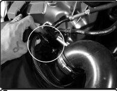
**7.** Disconnect the MAF sensor harness from the intake tube. Pull
