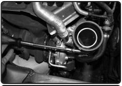
**12.** Tighten the clamp on turbo only.
