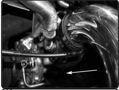
**19.** Secure the hose and tighten using 8mm nut driver.
