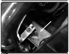
17. Once positioned, secure the bracket using provided M6 nut and fender washer. Secure and tighten using 10mm wrench or socket.
