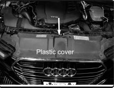
2. Front plastic cover needs to be removed for access to the air box scoop.
