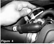
Carefully pull back the vacuum line from the stock intake tube.
