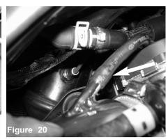
Attach the vacuum line to the fitting located on intake tube and secure.
