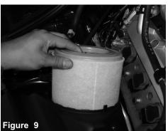
Now remove the filter out of vehicle.
