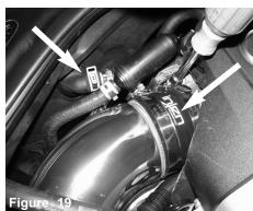
Tighten clamps on throttle body using 8mm nut driver.
