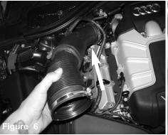
Pull back the vacuum line from the intake tube and remove the stock intake tube out of vehicle.
