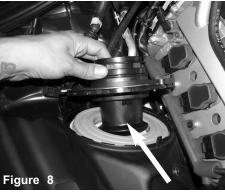
Remove the adaptor out of the vehicle.
