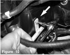
Locate the A/C bracket on the strut tower near firewall and loosen the screw using T30 torx bit. remove screw.
