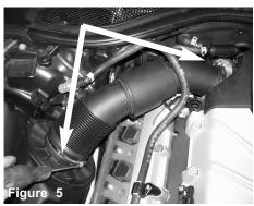
Loosen the clamp on the throttle body and air box side using 7mm nut driver.
