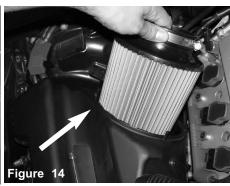
Attach the 3" hose with clamps provided to the intake
