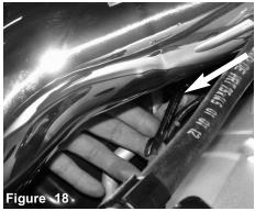
Position for best fit and tighten using 10mm wrench.
