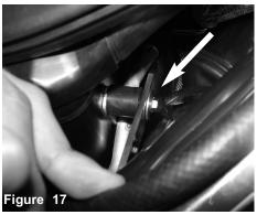
Secure the bracket to the vibra mount using provided fender washer and m6 nut.
