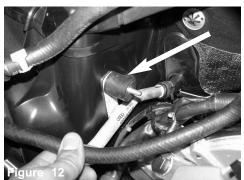
Tighten the vibra mount and secure.
