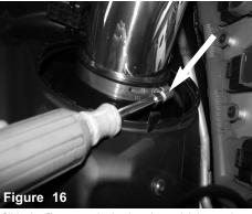
Slide the filter on to the intake tube and tighten using 8mm nut driver.
