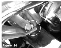
Secure the bracket using provided M6 washer and nut. Tighten the nut using 10mm wrench.
