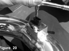
Secure the intake tube using the factory M4 screws.
