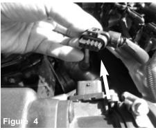
Disconnect MAF sensor harness and set aside.
