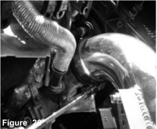
Tighten the remaining clamp using 8mm nut driver.
