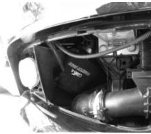
Install the air filter to the tube and tighten using 8mm nut driver.
