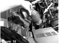
Remove the intake tube from the vehicle.
