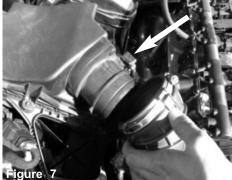
Pull back the factory intake tube.
