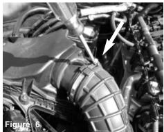
With flat head screw driver, loosen clamp.
