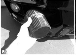
Attach the hydro shield to the air filter and install through Install the intake tube into vehicle. the bottom of the valence next to fog light. (if equipped) Set on bottom under head light up side down.
