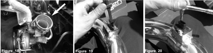
Install the step hose to the turbo and tighten the clamp on turbo only
