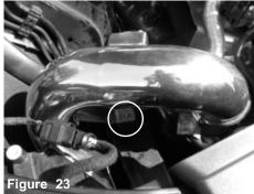
Position the intake tube to the step hose and the bracket to the stand off stud.
