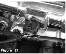
The harness plug is shown firmly pressed over the sensor clip.
