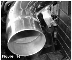
Align the intake bracket to the vibra-mount stud while the top end is pressed into the turbo inlet.
