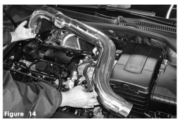
Align the pre-tuned intake system over the engine compartment.
