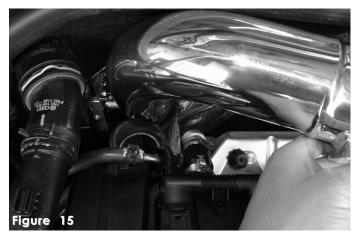
Insert the top end of the intake into the throttle body hose connected on the turbo inlet.
