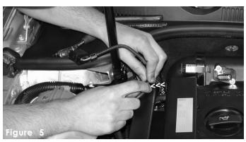
Remove or disconnect harness wire from the IC air cooling duct.
