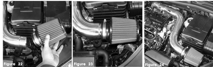
Take the tuned filter and press it over the end of the intake. Once the intake end has butted up against the filter stops, continue to tighten the filter neck clamp.
