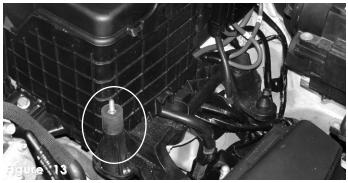
The vibra-mount is fully threaded into the mounting pad
