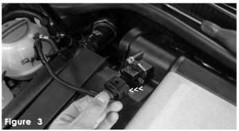
Disconnect harness plug from the sensor clip as shown above.
