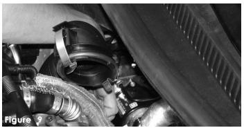
Loosen clamp on the turbo inlet. Once you have loosened the clamp, continue to remove the plastic elbow.
