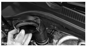
The plastic pressure fit elbow is still connected to the turbo inlet once the engine cover has been pulled out.
