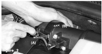
Loosen two metal clips on the pressure fit elbow that is inserted into the sensor housing (A) and (B).
