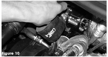
Press the 2 1/2" elbow over the turbo inlet until the hose is flush over the inlet.
