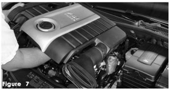
Once all plugs, clamps, and connectors have been removed, continue to pull the engine cover out of the engine compartment.
