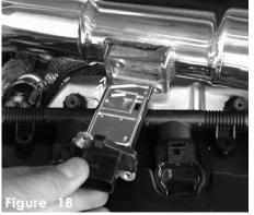
Insert mass air flow sensor into the machined sensor adapter.
