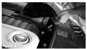
Remove the front plastic expanding plugs and torx bolt by the side battery base in order to detach the front air scoop.
