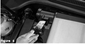
Unscrew two torx screws from the mass air flow sensor. Once screws have been removed, continue to pull the mass air flow sensor from the sensor housing.
