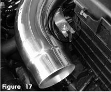
Once the intake bracket is lined up to the vibra-mount stud, use the m6 flange nut and fender washer to fasten the intake in place.
