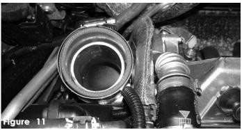
Once the hose is sitting flush on the turbo inlet, continue to place two .312 powerbands over the hose. Tighten band that is on the turbo inlet side at this point.
