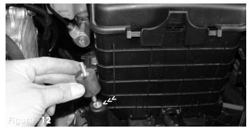
Align the m6 vibra-mount over the pre-threaded battery tray mounting pad.
