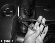
With pliers, pinch factory clamps and pull back stock intake tube from MAF sensor.
