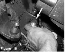
Locate hole underneath headlight and insert vibra mount stud through hole.
