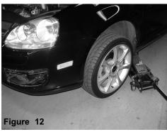
Jack front driver side of vehicle allowing enough room for filter installation.
