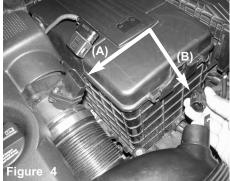
Disconnect electrical MAF sensor (A) and air Intake air temperature sensor(B).
