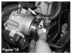
Press straight hose with clamps over the throttle body, tighten clamp over the throttle body at this point.
