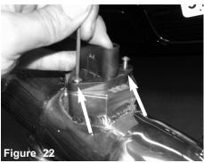
Insert the MAF sensor into new intake tube. Secure using provided M4 button head screws and tighten using 2.5mm allen key.
