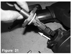
With tamper resistant bit or pliers, carefully remove the 2 screws holding in MAF sensor from housing. Remove sensor.
