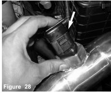
Re-connect the electrical MAF harness until you hear it snap together.
