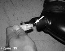
Remove the electrical temperature sensor from stock air intake duct.
