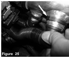
Re-connect the crank case and smog pump fittings to Align the intake for best fit and tighten clamp on the intake tube.
