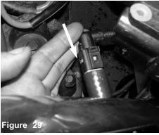
Re-connect the electrical temperature sensor
