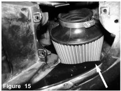
Place filter upside down and position. Secure splash guard to the original state and lower vehicle then remove jack.
