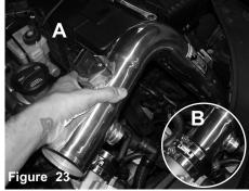
A) Lower the intake tube and align bracket to vibra
