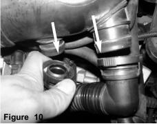
With pliers, pinch remaining clamp on throttle body and Disconnect the crank case and smog pump fitting clips A) With phillps, loosen screw holding in lower bumper from stock intake tube. Remove stock intake tube from
