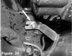
The intake bracket is aligned to the vibra-mount stud, using provided M8 nut and washer, tighten using a 12mm socket or wrench.
