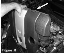
Remove factory air box/engine cover from the vehi-
