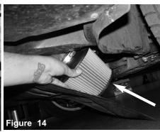
Place the air filter through bottom of vehicle, positioning it in front of bumper.
