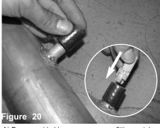
A) Press provided hose over vacuum fitting on tube. B) Carefully break the 3 fin-tabs on temparture sensor, now install to hose and secure. Note: Make sure sensor is pressed all the way inside, and partially in fitting also.
