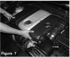
Carefully lift and pull up on the factory air box/engine cover and remove it from the engine.
