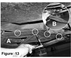
A) Get underneath front of the vehicle, with T25 torx key, loosen the 4 screws holding in splash guard on driver side only.
