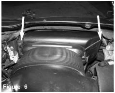
With T25 torx key, loosen the 2 screws holding in factory ram-air unit attached to the radiator support.
