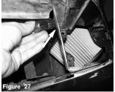
Press the air filter over the intake tube. Tighten using 8mm nut driver. Re-install lower bumper valence.
