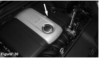
If your going to be using reusing the engine cover, you'll have remove ram air unit or front air scoop along with the MAF housing on the air intake box then re-install engine cover.
