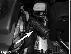
This is an auxillary heater hose line that picks up ambient warm air on cold starts. This will not be used with the injen intake kit.
