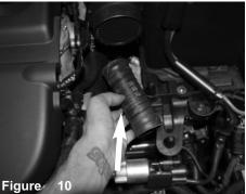
Carefully remove the heater hose from vehicle.
