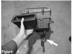
Now with the whole intake removed, this drain plug will not be used.
