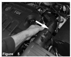
Rotate the MAF sensor towards the battery. This will unlock the bottom of the MAF sensor.
