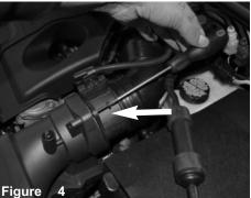
With T25 torx bit, loosen the 1 screw holding in MAF sensor.
