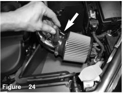
Install the filter to the intake tube and tighten using 8mm nut driver.
