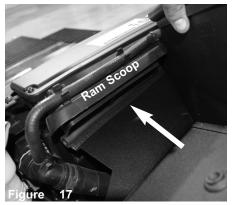
Install the front side with rubber trim underneath the factory Ram scoop first. Position the grommets to the factory OEM air box fittings.
