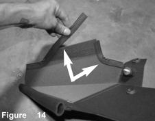
Now install the bulb edge trim to both sides of the top of the heat shield.
