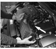
Lift up and remove the air box box from vehicle.
