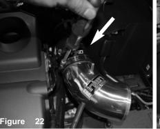
Tighten the clamp on the MAF sensor. Position for best fit.
