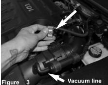
Disconnect MAF sensor harness. Disconnect and remove the small vacuum line.
