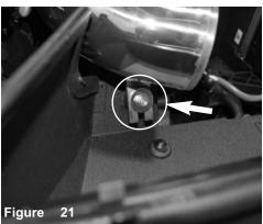
Secure the bracket using provided M6 nut and fender washer.
