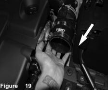
Install the 3-1/8" straight hose with clamps to the MAF sensor.
