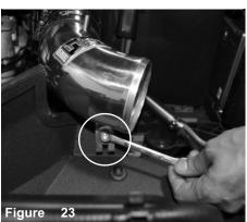
Position for the best fit, and tighten the vibramount using 10mm socket or wrench.
