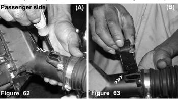
Removing the bolts from the mass air flow sensors: Use an 8mm nut driver to remove the 4mm bolts from the mass air flow sensors as shown above. Once you have removed the bolts, continue to pull the mass air flow sensor from the sensor housing, repeat the same steps on the driver side sensor housing.
