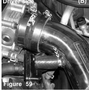
Installing the 17mm breather hose: You can either insert the 17mm hose over the CCV box port or the air intake port as shown in figures (A) and (B).
