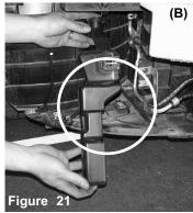
Looking down in front of the passenger side you'll notice a silver metal plate with three prongs. These clips are holding the plastic resonator box in place. Use a flathead screwdriver to dislodge the resonator box from the bracket (A). Bracket is shown in figure 24 below. Now, pull the resonator box out of the bumper area (B).
