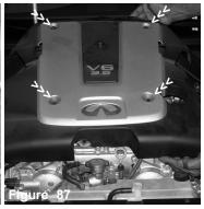
Replace the engine cover and secure it using the stock bolts.
