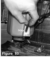
Connect the electrical wire harness clip to the top motor, you will hear it snap in place(A). Press the black line over the motor port as shown in figure (B). Note: The level indicator sensor is not used for this application because of possible leaking. The deletion of the level indicator sensor will not cause the "check engine" light to come on, be sure to zip tie it away in a safe place.
