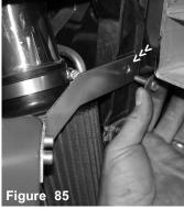
align the horizontal bracket to the mounting hole and use the stock bolt to fasten the bracket to the brace.
