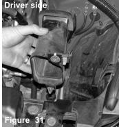
Once you have removed the bolt and the two plastic clips, the air scoop should pull right out. Above, passenger side and driver side air scoops are shown.
