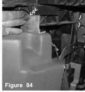
Once all lines have been connected, align the top bracket to the stock hole and use the stock bolt to secure it.
