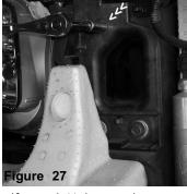
Removing the two front air scoops: Use a 10mm socket to loosen and remove the 10mm bolt on each of the front air scoops as shown above.
