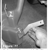
Use the m6 x 12mm bolts in this kit to fasten the bracket to the reservoir bottle (A). The horizontal long bracket is now aligned to the side m6 press nuts (B)
