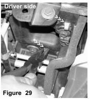
Continue the removal of the two front air scoops: Using a pair of needle nose pliers, compress the plastic clips together and push the clip in, this will release the air scoop from the crossmember. Do the same for the lower plastic clip then repeat the same steps on the driver side air scoop. Page 3 of Part# SP1997
