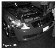
Place the bumper back to its original position and fasten it in place using all plastic clips and bolts that where removed.
