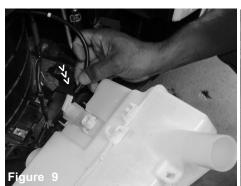
Disconnect the black hose connected to the motor .
