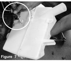
Prior to pulling the reservoir bottle out, pull the upper spout out of the lower spout. Depress the tab on the electrical harness and pull the clip away from the motor.
