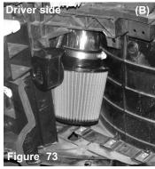
The Dyno-tuned filter is aligned and pressed over the end of the intake (A). The filter is pressed over the intake until it comes to rest against the built-in filter velocity stack stop (B). An 8mm nut driver is used to tighten the filter neck clamp.
