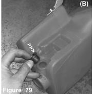
Use the last of the m6 x 12mm bolts to fasten the bracket to the reservoir bottle as shown in figure (A). The grommet that was removed from the stock reservoir bottle is now inserted into the new reservoir bottle (B).
