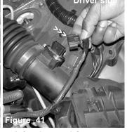
Depress the plastic tab and pull the harness clip from the mass air flow sensor.
