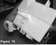
Prior to pulling the motor out, empty the contents into an empty container to be used with the Injen reservoir bottle. Pull the motor out from the rubber grommet.
