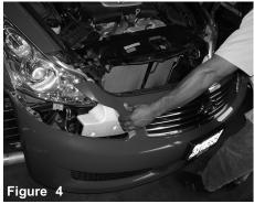
Remove all plastic clips and bolts holding the bumper in place. Once you have removed all clips and bolts, continue to pull the bumper away from the frame.
