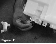
Pull the rubber motor grommet out of the reservoir bottle as shown above
