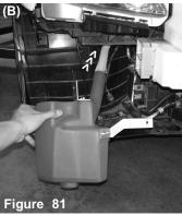
Once you have pressed the stock grommet into the pre-drilled hole, continue to press the motor into the grommet (A). Place the assembled reservoir bottle into the front bumper section and push up into the engine compartment (B).
