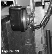
The horn is now completely installed towards the front of the bumper. Picture (A) shows the front and picture (B) shows the back.
