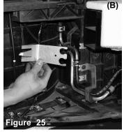
The bracket on the passenger side is held on grommets, pull the silver metal bracket out as shown in figures (A) and (B), this will allow additional room for the filter and new reservoir bottle. The drive side bracket will remain in place.
