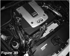
Align the intakes for best possible fit. Once you have aligned and made sure that the length of the intakes are free from any moving parts, continue to tighten all nuts, bolts and clamps.
