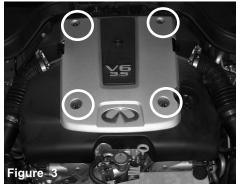
Loosen and remove all four 10mm bolts from the engine cover. Once all bolts have been removed, continue to pull the cover from the engine compartment.
