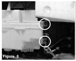
Remove the last two remaining 10mm bolt from the side of the reservoir bottle.
