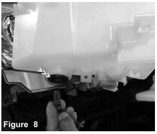
Pull the electrical harness clip away from the sensor as shown above. This electrical harness will not be used with the Injen reservoir bottle.
