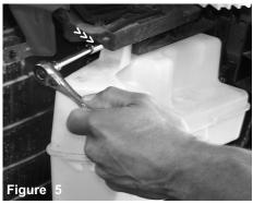
Once you have removed the bumper, continue to remove the windshield reservoir bottle. Remove the first 10mm bolt as shown above.
