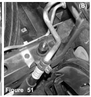
Align the composite stand-off over the stock grommet (A) push down on the stand-off until it is fully inserted into the grommet (B)...
