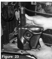
Repeat the same steps on the driver side as you did on the passenger side. Lift the center pin using a flathead screwdriver (A) and pull the resonator box out of the front bumper (B).
