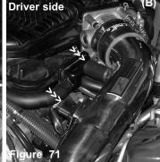
The 17mm stub and electrical harness clip are now installed on both the passenger and drivers side.
