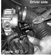
Once the CCV box has been remove, continue to detach the air intake duct form the throttle body.
