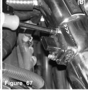
The same steps are repeated on the driver side, the mass air flow sensor is inserted into the machined sensor adapter A) and the stock 4mm bolts are used to fasten the sensor to the sensor adapter (B).
