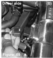
Align the harness clip to the mass air flow sensor and press the male clip over the female connector until it snaps in place. Repeat the same procedure with the harness clip on the driver side.
