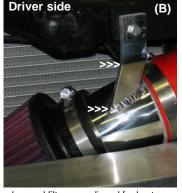
The passenger side and driver side filter couplers and filters are aligned for best possible fit, Once you have aligned the silicone intake hose, filter couplers and filters, continue to tighten the bolts and clamps. NOTE: Bend direction on brackets and angle cut on brackets to determine proper position of filter couplers.
