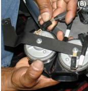
The second horn is aligned and attached to the top of the new bracket, the nut is used to secure the horn in place (A). The electrical wires are reconnected as shown above (B).
