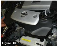
The lower engine cover is aligned to the upper engine cover as shown above. Use the 2-10mm flange nuts and the 2-10mm bolts to fasten the engine cover in place
