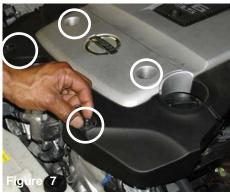
Removing engine covers: Remove the 2- 10mm flange nuts and the 2-10mm bolts from the lower engine cover.
