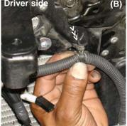
Depress the plastic tab and separate the male and female harness clips (A), pull the male clip away from the crossmember, this will allow the harness to be extended (C). Pull the plastic clip on the wire loom from the crossmember to allow wire harness to be extended further down into the bumper area (B).
