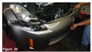
Remove all six plastic clips from the upper bumper area and all 14- 10mm bolts from the lower bumper area. Once all clips and bolts have been removed, continue to pull the bumper away from the car.
