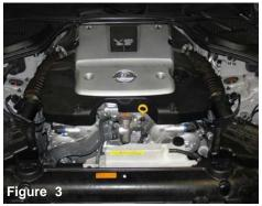
Stock air intake cleaner and air ducts shown in this picture. Before getting started with the installation, disconnect the negative battery terminal and remove the strut tower bar from the engine compartment.
