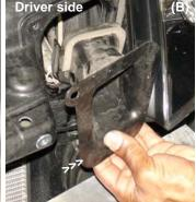
Remove the plastic clips from the front air scoops which are located in front of the passenger side (A) and the driver side (B) cross member.
