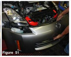
The front bumper is now replaced and all bolts and plastic clips are used to fasten the bumper in place.
