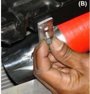
The driver side filter coupler is pressed into the end of the silicone intake (A). The coupler bracket is aligned to the m6 nut on the bumper bracket, use the 10mm bolt to fasten the coupler in place (B).Note: must use driver side coupler
