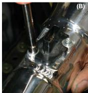
The driver side mass air flow sensor is lowered into the billet machined sensor adapter (A). Once the mass air flow sensor has been carefully positioned in place, continue to use the stock bolts to secure the mass air flow sensor in place (B).
