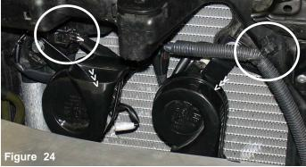
Stock horns to be removed and relocated. Circled above are the harness clip and wire loom that need to be removed from the crossmember, this will allow the harness and horns to be relocated into the lower bumper area.
