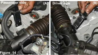
Once all bolts have been removed from each of the mass air flow sensor, continue to pull the mass air flow sensors from the passenger side (A) and the driver side (B) air intake ducts as shown above.
