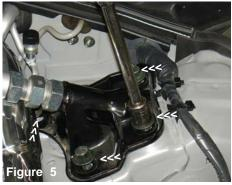
Remove the 3- m14 bolts and 1- flange nut located on the drive side strut bar bracket.
