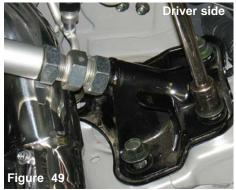
The 3- 14mm bolts and single 14mm nut is use to fasten the driver side bracket in place.
