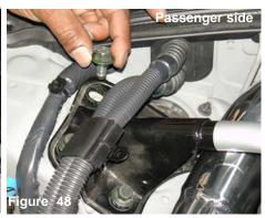
The 3- 14mm bolts and single 14mm nut is use to fasten the passenger side bracket in place.
