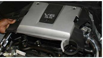
The upper engine cover is re-installed to its stock location as shown above. Use the 2-10mm flange nuts and 1-10mm bolt to fasten the upper engine cover in place
