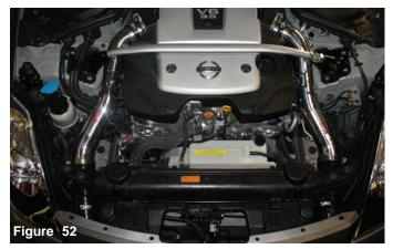
Align the entire intake for best possible fit. Once you have aligned and made sure that the length of the intake is free from any moving parts, continue to tighten all nuts, bolts and clamps.
