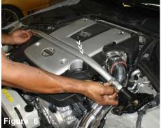
Once all 6- 14mm bolts and two flange nuts have been removed, continue to pull the strut tower bar out of the engine compartment,
