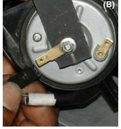
The first horn is aligned and attached to the new bracket, the copper connectors are re-attached prior to securing it with the nut (A). The copper connector is reattached and the electrical wires are reconnected as shown above (B).
