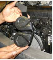
The electrical wires are all reconnected to the horns and the horns are secured to the new bracket(A). The horns are now ready to be lowered behind the bumper area (B).
