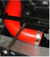
The new passenger side bumper bracket is aligned to the stock location (A), use the stock 10mm bolt to fasten the bracket in place (B).
