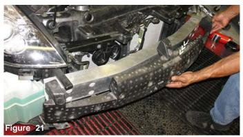
Remove the foam bumper padding from the aluminum bumper support as shown above.
