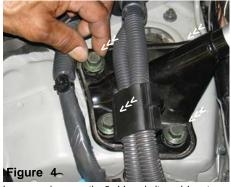
Loosen and remove the 3- 14mm bolts and 1- nut shown on the passenger side.
