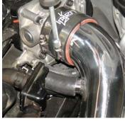
The 1 1/2" long, 15.9 mm hose is pressed over the air intake port (A) The 15.9 mm stub can also be pressed over the CCV box as well. The 15.9 mm stub on the air intake port is now pressed over the CCV box port (B). Insert the upper intake into the throttle body hose, adjust and use an 8mm nut driver to semi-tighten the clamp.
