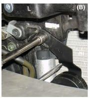
The assembled horns and bracket are now lowered behind the bumper area and attached to the driver side stock location. The stock 10mm bolt is used to fasten the horn bracket in place (A), A 10mm socket is used to fasten the horn bracket in its original location.
