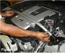
set the strut bar over the engine cover and align the brackets to the strut tower mounts. Use the 6-14mm bolts and 2-14mm nuts to secure the strut bar in place.
