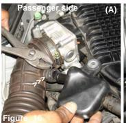
Use a per of pliers to depress the tension clamps on the air intake ducts. Once the tension clamps have been depressed, continue to pull the crankcase air ventilation boxes from both passenger side (A) and driver side (B) air intake ducts.
