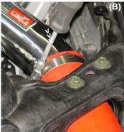
The power-bands are placed over the 90 degree silicone intake hose (A), the upper end is inserted into the driver side front air scoop opening (A) the silicone hose is pressed over the intake end (B), adjust and tighten the clamp on the silicone hose (B)
