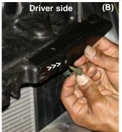
Remove the 10mm bolt from the bumper bracket as shown above. Once the bolt has been removed, continue to remove the brace from the passenger side (A) and driver side (B).
