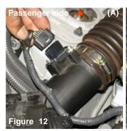
Depress the side locking tab on the electrical harness clip and pull up on the harness clip as seen on both (A) and (B).
