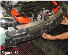
The foam bumper insulation is replaced in front of the aluminum bumper support.
