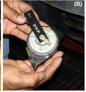
Remove the 10mm bolt holding the passenger side horn (A) The electrical wires are disconnected from the passenger side horn, the nut is also removed in order to separate the horn from the bracket (B).
