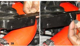
The new driver side bumper bracket is aligned to the stock location (A), use the stock 10mm bolt to fasten the bracket in place (B).
