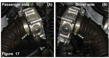
Loosen both hose clamps on the passenger side (A) and driver side (B) air intake ducts.
