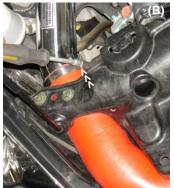
The power-bands are placed over the 90 degree silicone intake hose (A), the upper end is inserted into the front air scoop opening (A) the silicone hose is pressed over the intake end (B), adjust and tighten the clamp on the silicone hose (B)
