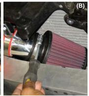
The Dyno-tuned filter is aligned to the passenger side filter coupler (A). The filter is pressed over the coupler until it comes to rest against the built-in filter velocity stack stop (B). The 8mm nut driver is used to tighten the filter neck clamp (B).
