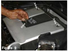
Loosen and remove the 2-10mm flange nuts and 1-10mm bolt from the upper engine cover as shown above.
