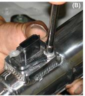
The passenger side mass air flow sensor is lowered into the billet machined sensor adapter (A) . Once the mass air flow sensor has been carefully positioned in place, continue to use the stock bolts to secure the mass air flow sensor in place (B).
