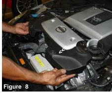
Once all nuts and bolts have been removed, continue to pull the lower engine cover out of the engine compartment.
