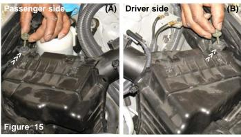
Remove one m6 bolt from the passenger side (A) and driver side (B) air box cleaner. A single bolt secures each air box cleaner in place.
