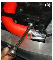
The passenger side filter coupler is pressed into the end of the silicone intake (A). The coupler bracket is aligned to the m6 nut on the bumper bracket, use the 10mm bolt to fasten the coupler in place (B). **Note: must use passenger side coupler**
