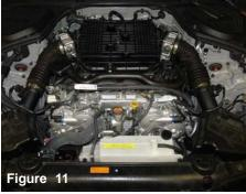
The two piece engine cover has been removed from the engine compartment. The air intake ducts and air box cleaner are now ready to be removed.
