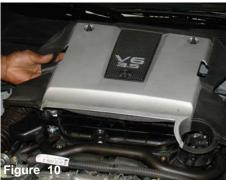
Once all nuts and bolts have been removed, continue to pull the upper engine cover out of the engine compartment.
