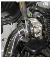
The 1 1/2" long, 15.9 mm hose is pressed over the CCV box port (A) it can also be pressed over the intake port as well. The 15.9mm stub on the CCV box is now pressed over the air intake port(B). Insert the upper intake into the throttle body hose, adjust and use an 8mm nut driver to semi-tighten the clamp.
