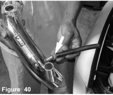
Press the 10mm hose over the intake vacuum port until it covers 75% of the vacuum port.
