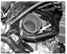
Press the silicone step hose over the turbo inlet and use two .048 power-clamps on the step hose. Tighten the clamp located over the turbo inlet.
