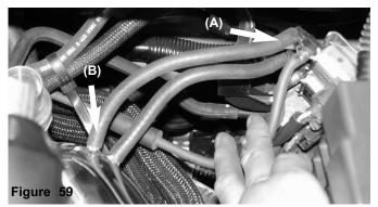
Once the 6 3/4" hose has been pressed over the upper solenoid port (A) continue to press the other end over the intake port (B). **Note:** The splitting of the lines will increase your boost thereby, given you faster response time.
