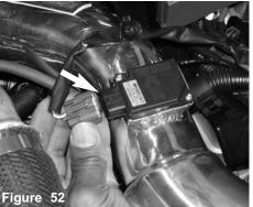
Align and connect the electrical harness to the mass air flow sensor.
