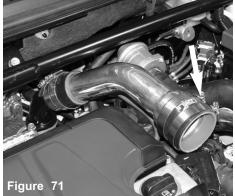
Once the hose has been installed, continue to tighten the clamp over the tubing.
