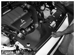
If the upper intercooler tubing is going to be replace con-tinue with figure 17 thru 23. Remove all plastic clips from the plastic shroud and remove the front shroud as shown above.
