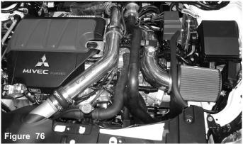
Top shot of the complete installation with the intercooler piping.
