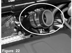
Press the 2" x 2 1/2" long straight hose over the upper intercooler inlet, use two .032 power-bands on the straight hose. Tighten the clamp on the inlet side for now.
