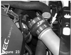
Press the 2 1/2" hump hose over the lower intercooler outlet, use two .040 power-bands on the hump hose, Tighten the clamp on the outlet tube for now.
