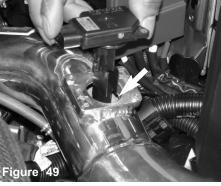
Carefully insert the mass air flow sensor into the machined sensor adapter. We recommend you apply a small of amount of light oil on the O-ring to prevent any kinking or tearing.
