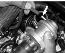
Once you have pulled the BOV from the air intake port, remove the 4mm vacuum line from the BOV port.
