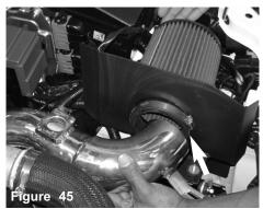
The filter neck base is pressed over the inlet side of the intake.
