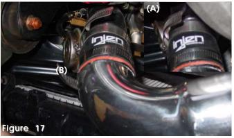
Press the 1.75" X 2.00" Step hose over the turbo inlet, use one small .024 power clamps, tighten the clamp on the turbo inlet at this time (A). Insert the 2" side of the hot pipe into the 2" hose and semi-tighten the power-clamp (B).
