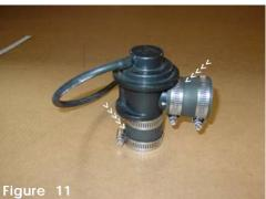
Press the new reinforced short hose over each port on the blow-off valve. Use the .020 mini clamps provided in this kit to secure the hose in place.
