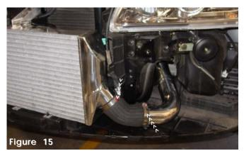
Two .312 bands are used to connect the secondary intake to the intercooler tank. Injen now sells massive bolt-on intercoolers kits for the 2003-06 EVO VIII, MR, and EVO IX. Size 23 1/2""x11 3/4" x 3 3/8"
