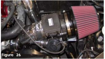
Press the assembled mass air flow sensor and filter over the end of the cast intake. Position for best clearance and tighten the clamp.
