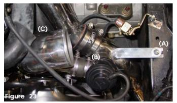
Top view of the bracket (A), blow-off valve (B) and cast intake (C) all connected and ready for the next step.
