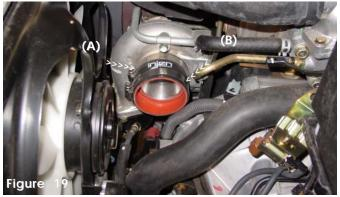
Press the 2 1/2" x 3" step hose over the turbo and use one .312 small power- band on the turbo and tighten the clamp (A). Place one .362 power-band on the other end of the hose but do not tighten yet (B).
