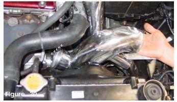
Insert the cast intake into the step hose on the turbo inlet . Position the intake and semi-tighten the clamp. Page 3 of Part# SP1898
