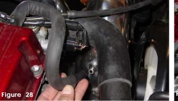
Press the stock crankcase hose over the 3/8" nipple on the intake. Make sure it is properly fitted, clean any excess oil in the line to prevent the hose from slipping off. Page 4 of Part# SP1898
