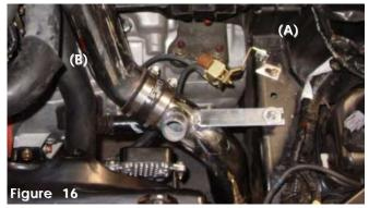
The secondary intake bracket will align to the vibra-mount stud(A). Use the m6 nut and washer to hold the intake in place. Insert to top end into the 2 1/2" hose and align the intake before you semi-tighten any of the clamps (B).
