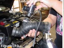
Remove the blow-off valve from the stock intake duct.
