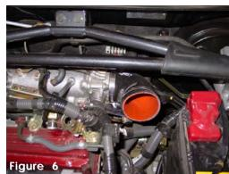
Press the 90 degree elbow on the throttle body and use two power-bands on the elbow. Semi-tighten the clamp on the throttle body at this time.
