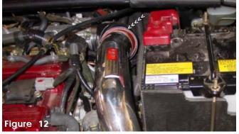
Insert the primary intake into the 90 degree throttlebody elbow, and use two clamps. Align the intake and semi-tighten the clamps.
