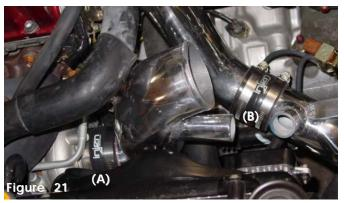
The cast intake (A) and secondary pipe to the intercooler (B) has been installed and ready for the next step.
