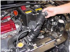
Remove the stock air intake duct connected at the throttle body (A) and the air intake box (B).
