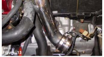
Press the 2 1/2" straight hose over the end of the intake and use two power-bands, tighten the band on the intake.
