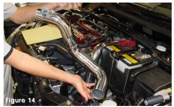
Take the secondary intake tube and lower it into the bumper section. Insert the lower end into the intercooler stock elbow but do not tighten any clamps until the intercooler tubing has been aligned. (See figures 15 & 16)
