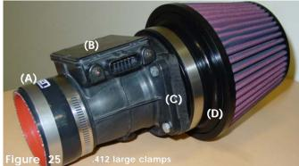
Press the 3 1/4" hose (A) over the end of the air sensor (B), place two power-bands over the hose. Butt the composite flange up to the the air sensor and use four m6 x m25 bolts (C). Press the filter over the end of the composite flange and tighten the filter clamp (D)
