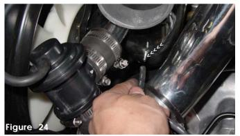
The 4mm return stock return line is connected to the small port on the intake. Note: Be sure to reuse the stock clamps on the 4mm line.
