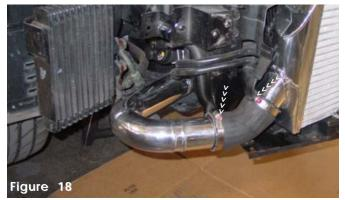
Insert the 2 1/2" end of the hot pipe into the intercooler elbow and replace stock clamps with the two power bands.
