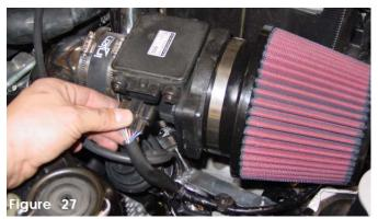
Press the harness clip into the mass air flow sensor until you hear a sharp snap. Be sure to reconnect the sensor before moving on to the next step.
