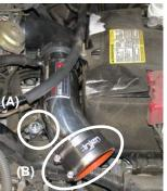
Use the 6mm flange nut and fender washer to secure the intake to the vibra-mount (A). Press the 3 1/4" hose over the intake, use two clamps and tighten the clamp on the intake (B).
