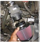
Press the 3 1/2" filter neck over the end of the composite flange.
