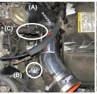
Once the intake has been pressed into the elbow on the throttle body (A) Align the intake bracket to the vibra-mount stud (B). Press the stock vacuum line over the intake port (C).
