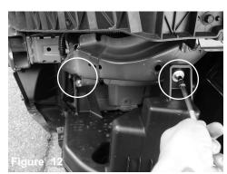
Loosen the 2 bolts holding in the resonator box.
