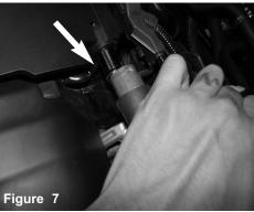
Pull the crank case line away from the engine fitting.
