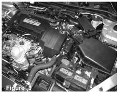
Stock air box shown in this picture, disconnect battery before installation.
