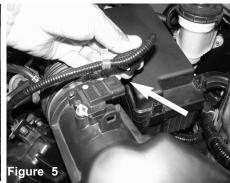
Disconnect the MAF sensor harness and pull the line away from the air box.
