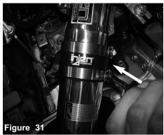
Secure and tighten the clamps on filter.
