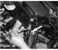
Use a 10mm socket and rachet and remove the 10mm bolt connecting the ECU bracket to the battery support bracket.
