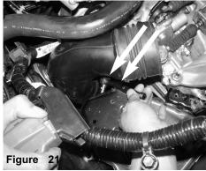
Remove the two 10mm bolts attaching the lower air box resonator duct to the battery support bracket.
