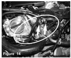
Now connect the other coolant line from the upper radiator hose housing to the coolant line hose from the throttle body.
