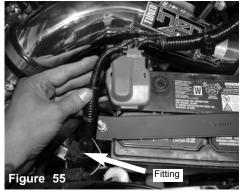
Disconnect fitting on radiator support holding in Positive line. Install the positive terminal to battery and position for clearance in tube. Tighten using 10mm.
