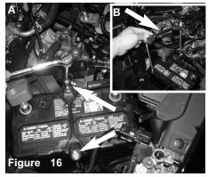
Figure A: Loosen the 10mm nuts on the battery tie down. Figure B: Unhook the battery tie down hooks from the frame and then remove from engine bay.,
