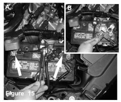
Figure A: Loosen the 10mm nuts on the positive and negative battery terminals. Figure B: Detach both battery terminals from the battery.
