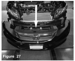
Remove the bumper cover. Remove the 2 phillips screws on side. Remove the 2 push clips on top and remaining push clips on bottom.
