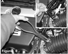
Figure A: Use a set of needle nose pliers and release the pressure on the tension clamps. Figure B: Pull the metal crank case vent tube (CCV) out of the rubber intake duct.
