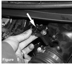
Pull the MAF sensor out of the air box housing
