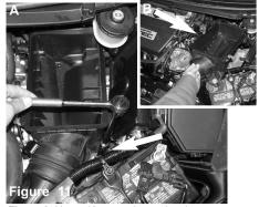
Figure A: Use a 10mm socket and rachet to remove the bolt on the front right side of the lower air box assembly. Figure B: Lift up on the back side of the lower air box assembly to detach the rear grommets and then pull the lower box assembly out.
