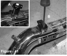
Figure A: Install the MAF sensor into the tube. Figure B: Secure the MAF sensor using factory screws. Tighten using phillips screwdriver.
