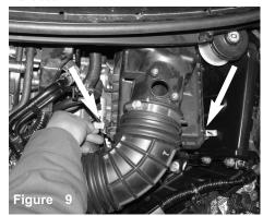
Unclip the two clips attaching the upper and lower air box assemblies together.
