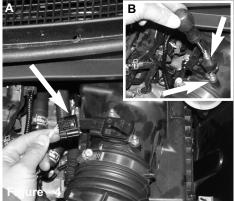
**Figure A:** Disconnect the MAF sensor harness. **Figure B:** Use a phillips screw driver and remove the two screws on the MAF sensor.
