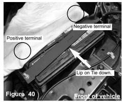
Tighten the battery using 10mm deep socket. Make sure the battery is centered between the thredded straps. Make sure the battery is not touching anything.
