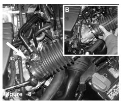
Figure A: Use a 10mm socket and rachet to loosen the clamp on the rubber air duct connected to the throttle body. Figure B: Pull the rubber duct off the throttle body
