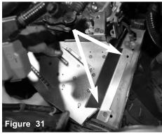
Slide the 2 tabs in the 2 bolts from previous step. The remaining 2 holes line up the top holes on vehicle frame.
