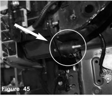
Secure and tighten using 12mm socket and ratchet.
