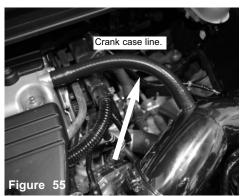
Install the provided 15mm crankcase hose to the engine fitting and fitting on intake tube. Re-install the bumper cover.
