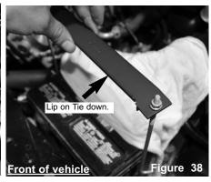
Now install the thredded fitting straps to the new injen battery tie down. Note: Make sure that the side with the 1/4" lip is facing front of vehicle.
