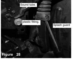
Locate the sound tube on resonator. With a flathead, remove the rubber hose from the resonator. Inside the fender well on splash guard, remove the plastic push clip holding on the resonator.
