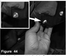
Install the vibramount into the hole. Secure using provided M8 nut and washer.
