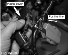
If desired, you can remove the positive battery line cover from line. This will allow for more clearance.
