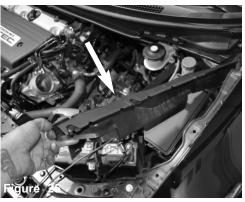
Remove the plastic side cover inside the engine compartment. Release the push clips to remove.
