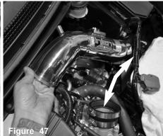
Install the upper intake assembly into the vehicle.
