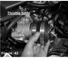
Install the step hose with clamps to the throttle body. Make sure the 2-7/8" side is on the throttle body.
