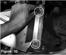
Now secure the top of the new battery bracket. Secure using the factory bolts. Tighten these 2 first, Than tighten the bottom 2 from step 30 last. Secure using 12mm socket and ratchet.
