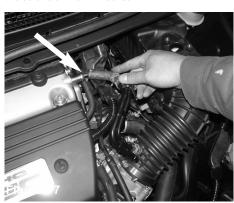
Now remove the rubber line connected to the CCV port on the valve cover.
