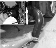
Install the 90 silicon hose with clamps provided from the bottom up. Make sure the side with injen logo is on top. Position for remainder of installation.
