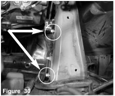
From step 22, loosen the 2 bolts on frame. Do not loosen the bolts completely. Install the new Injen battery bracket into vehicle.
