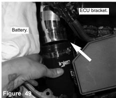
Now attach the 90 degree hose to the upper part of the intake assembly. Do not tighten.
