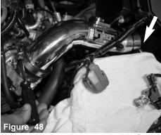
Make sure the tube on the step hose is sitting flat and all the way inside the tube. Tighten clamp. Make sure there is clearance between the battery and ECU bracket. Adjust if needed.
