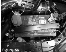
Verify in above image all circled have proper clearance and are not touching. Note: Injen Technology is not responsible or liable for damage to battery or intake system and will not be covered under warranty for inproper installation or clearance issues.
