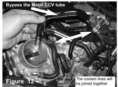
The metal CCV tube will need to be removed. Please note the routing of the coolant line that is connected to the throttle body to the upper radiator hose housing. The metal CCV line will be bypassed and removed and the two coolant lines will be connected together.
