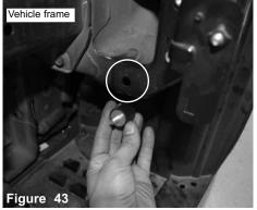
Locate the hole on the frame near air bag sensor.
