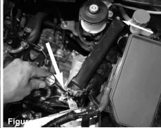
Now secure both bolts using 10mm socket and ratchet.
