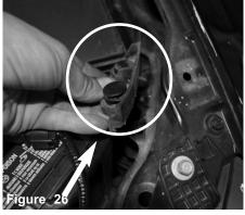
Remove the push clips and remove the smaller plastic cover.
