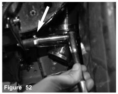
Secure the bracket using provided 12mm socket and ratchet.
