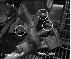
Locate the three 10mm bolts holding in the resonator. Loosen and remove. Carefully pull of the resonator from the vehicle.
