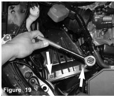
Use a 12mm socket and rachet and remove the two 12mm bolts on the battery support bracket attached to the chassis
