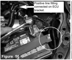
Rotate and position the negative terminal like above image and tighten using 10mm. Make sure the bracket tie down fitting is secured like above image. Verify hood closes and adjust if necessary.
