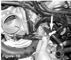
Place the supplied 1/4" plastic coupler onto the throttlebody coolant line.
