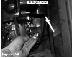
Install the lower intake assembly tube into vehicle. Make sure the non-beaded side is installed in the 90 degree hose. Position the bracket to the vibramount.
