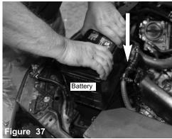
Now, install the battery into vehicle. Note: With a shop rag or towel, cover the terminals to prevent any contacts.
