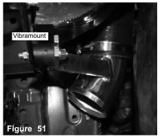
Position like above image. Secure the bracket using provided M8 nut and washer. Do not tighten.
