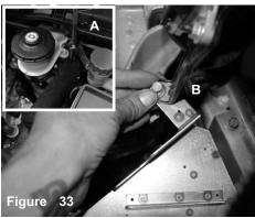
Figure A: Loosen the 10mm bolt on the ECU bracket. Figure B: Now secure the bottom of the bracket from step 20 using factory bolt.
