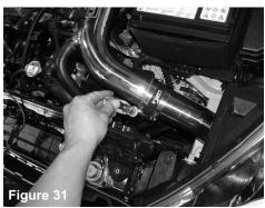
Adjust the entire intake system for best fitment. Make sure the intake pipe and filter does not come into contact with any objects and then continue to tighten the clamps on the 3.0" straight hose attached to the primary and secondary pipes.
