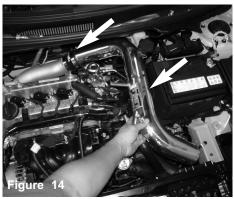
Position the intake pipe into the engine bay and place the end of the pipe into the steop hose on the turbo compressor outlet.
