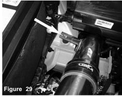
Attach the secondary intake pipe bracket to the vibramount on the chassis from figure 26. Place a supplied fender washer and M6 nut onto the vibramount and secure the bracket to the vibra mount.
