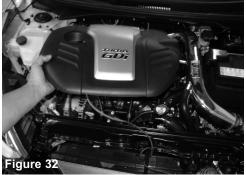
Reinstall the engine cover. Your intake installation is now complete. Go over all your clamps and fittings to make sure they are snug. Check the clearance on the pipe and make sure it does not make contact with any components in the engine bay.
