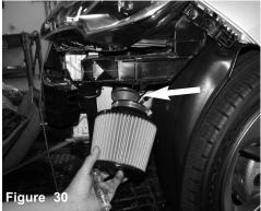
Place the filter onto the end of the intake pipe located in the bumper cavity. Use a 8mm nut driver and secure the filter clamp to the intake pipe
