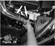
Attach the secondary tube from the bumper cavity to the primary intake pipe with the 3.0" straight hose
