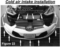
To continue with the installation of the cold air intake system, you will have to remove the front bumper by removing all the plastic retaining clips and screws indicated by the arrows in the photo.
