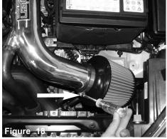
Place the filter onto the end of the intake pipe and then secure the filter to the pipe with a 8mm nut driver.
