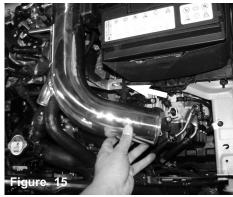
Line up the intake bracket to the vibra mount in figure 13
