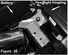
Screw the second vibramount mount into the threaded hole located on the chassis beneath the back of the driverside headlight housing inside the engine bay. Use the headlight housing and battery location in the photo for reference
