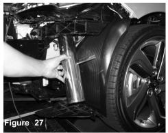
Slip the Injen secondary intake pipe up from the bumper cavity into the engine bay
