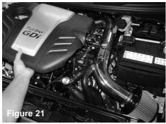
Reinstall the engine cover. Your short ram intake system installation is now complete. Go over all your clamps and fittings to make sure they are snug. Check the clearance on the pipe and make sure it does not make contact with any components in the engine bay.
