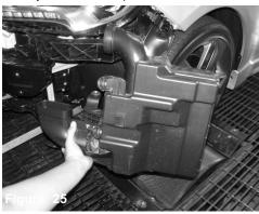
Remove the entire air box resonator from the bumper cavity.
