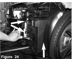
Remove the three 10mm bolts attaching the air box resonator located in the drivers side bumper cavity to the chassis
