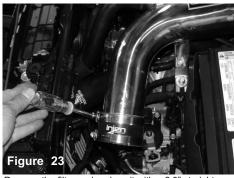
Remove the filter and replace it with a 3.0" straight hose and two #48 clamps
