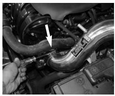
Secure and tighten clamp on throttle body using 8mm nut driver
