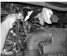
Use a plier to release the pressure clamp on the brake booster vent tube and then disconnect the booster vent tube from the air duct. NOTE: Manual models will not have this vacuum line.
