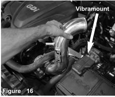
Figure A: Install the intake tube into vehicle and position to the straight hose and bracket to the vibramount.
