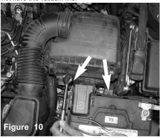
Use a 10mm socket and 3/8" rachet and extension and loosen the two 10mm bolts attached to the front of the entire air box assembly from the engine bay. the OEM air box assembly
