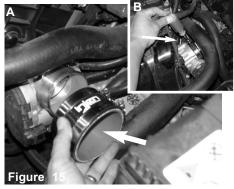
Place the 3.0" straight hose and two #48 clamps onto the throttle body. <u>Figure B:</u> Use a 8mm nut driver and secure only the clamp on the throttlebody side only for now.
