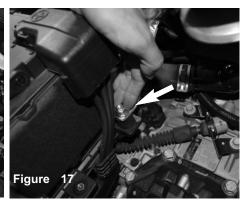
Now secure the bracket using provided M6 nut and fender washer.
