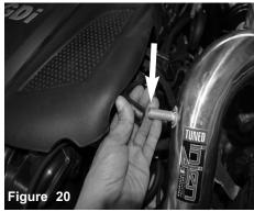
Connect the crank case line to the fitting on the intake tube.
