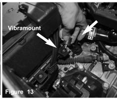
Now install the provided M6 vibramount behind battery in the airbox location insert.
