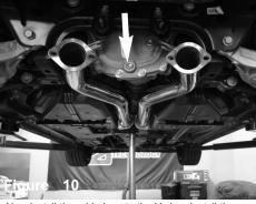
Now install the mid-pipes to the Y-pipe. Install the hangars to the rubber isolation mounts. Secure using provided 3" gaskets and bolts with nuts. **Do not tighten.**
