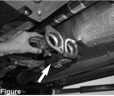
With exhaust removed, now install the adaptors with provided band clamp to the cat back. Make sure the slot cut out matches to the fitting on the stock down pipes. Tighten band clamp using 17mm socket or wrench. Position like above image.
