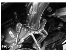
Snug fit all bolts and nuts using 14mm socket or wrench. Adjust for clerance and fitment. Make sure tips are centered of exhaust hole cut-out on bumper. Re-adjust if necessary. Use and extra hand for position of muffler and tighten all bolts and nuts.
