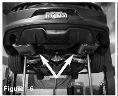
Carefully position and slide back and remove the exhaust out of the vehicle
