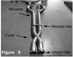
Make sure the x-pipe is installed on correct side. Look for labels on the x-pipe and fit with correct side only. With gaskets, install the x-pipe to the adaptors. Secure using provided M10 hardware. **Do not Tighten.**
