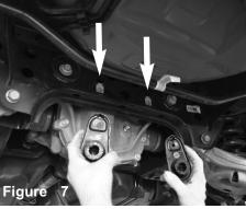
Remove the hangers from the factory exhaust. Use lubrication for easier removal. Re-install the rubber isolation mounts to vehicle and secure.
