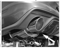
Install the rear section. Install the hangars to the rubber isolation mounts.
