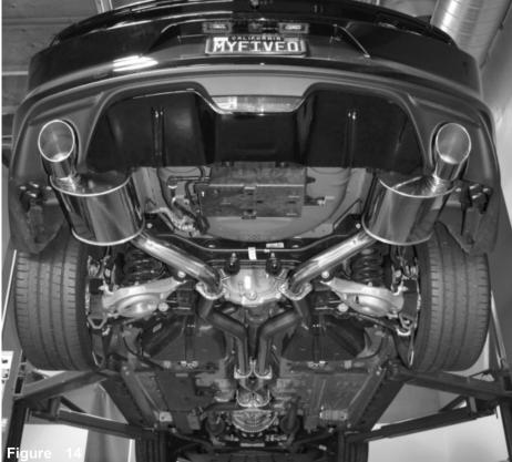
Congratulations! You have just completed the installation of this exhaust system. Periodically, check the alignment of the exhaust, normal wear and tear can cause nuts and bolts to come loose. <u>Note: Check clearance and adjust if needed! Failure to check the alignment and adjust the exhaust can cause damage that will void the warranty. Injen Technology is not responsible for any damages caused by/from improper installation.</u>
