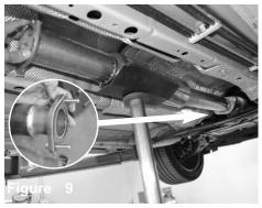
Re-use the factory gasket from step7, install the mid pipe to the factory catalytic converter flange. Secure using provided M8 bolt and nut. **DO NOT TIGHTEN!**
