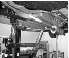
Remove the complete exhaust system out of the vehicle
