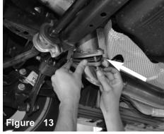
Secure flanges using provided gasket and M8 bolts and nuts. **DO NOT TIGHTEN!**
