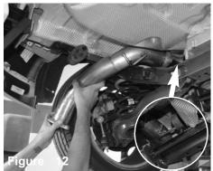
Install the 3rd pipe into vehicle and position the hangar to the factory rubber isolator.
