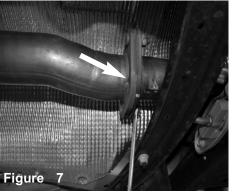
Loosen the 2 nuts on the flange using 15mm wrench. Save the factory gasket for new exhaust system. .
