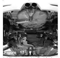
Your installtion is now complete. Check for clearance and position for best possible fit. Re-install the midframe support brace. Make sure there is clearance and the exhaust is not touching.
