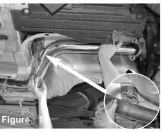
Install the 2nd pipe to the vehicle and position the flanges. Install the hangar into the rubber isolator.
