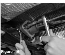
**Now position for the best fit,** This may require to loosen and retighten other flanges. Tighten all flanges using 14mm socket and wrench.
