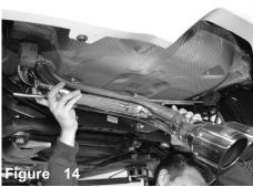
Install the final 4th piece into the vehicle. Position the flanges. Position the hangars to the rubber isolator.
