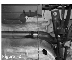
Locate this spot on the factory exhaust, this is a great spot to cut and also, if needed to re-install, you can have welded to have stock exhaust installed.
