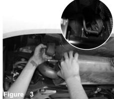
Lubricate all hangar isolators and pull back
