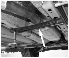
With 10mm socket and ratchet, loosen the 2 bolts holding in the mid-frame support brace, and remove.
