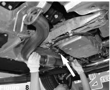
Install the Front section to the OEM downpipe.
