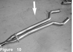
Now install the mid-pipes to the Y-pipe. Position for easier installation. This can be installed 1 piece. *Do not Tighten.*
