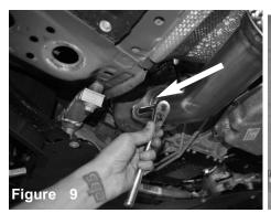
Secure using the OEM nuts. Do not Tighten.
