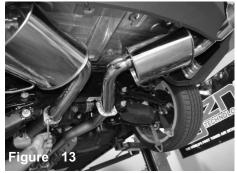
Snug fit all bolts and nuts using 14mm socket or wrench. Adjust for clearance and fitment. Make sure tips are centered of exhaust hole cut-out on bumper. Re-adjust if necessary. Use and extra hand for position of muffler and tighten all bolts and nuts.
