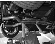
Install the mid assembly. Install the hangars to the rubber isolation mounts.
