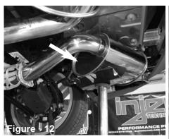
Install the rear muffler sections. Secure using provided 3" gaskets and bolts with nuts. **Do not tighten.**
