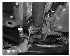
OEM exhaust system. Secure vehicle on lift. Loosen the 2 15mm nuts on OEM down pipe flange. Loosen and pull back.
