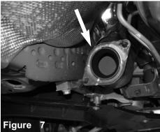
Make sure the OEM gasket is still used for new injen exhaust.
