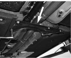
Loosen the 5 bolts holding in support bracket. Remove bracket for removal of exhaust and installation.
