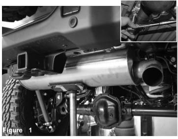
Remove the stock muffler using 15mm socket and wrench. Remove the hangars from stock isolators. Install the new Injen Axle Back Exhaust. Position the hangars to the stock isolators. Use Provided #63 torsion clamp in the kit. Position for the best to have access to the 17mm nut on clamp. **Do not tighten.** Install the Chrome tips to the exhaust adjust and fit to desired position and tighten.
