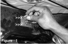
Line up the new plate hanger to the center of the rear axle and use the two m8 bolts.
