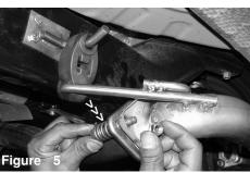
align the flange to the stock donut flange and use the stock spring loaded bolts and m10 nuts supplied.
