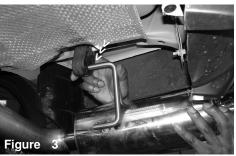
Raise the axle-back in place and insert the first hanger on the existing rear grommet.
