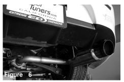
Align the entire axle-back for best fit and tighten the nuts and bolts, keep tip away from the bumper.
