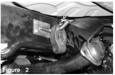
The hanger is installed and one of the unused grommets is re-hung on the hanger.
