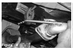
Push the second hanger near the flange into the second grommet as shown above.
